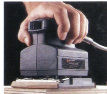
Double-insulated tools have non-conductive plastic bodies to prevent shocks caused by short circuits. Because of these features, double-insulated tools can be used safely with ungrounded receptacles
