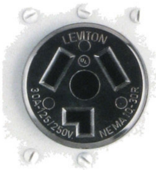
30 amps, 125/250 volts. This receptacle is used for clothes dryers. It provides high-voltage current for heating coils and 125-volt current to run lights and timers.
