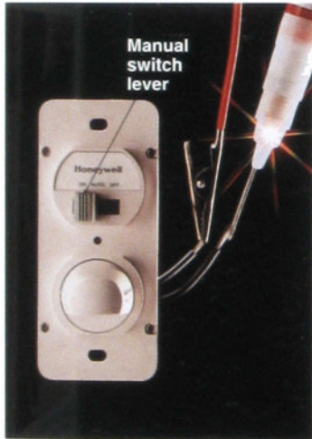
Automatic switch: Attach the tester to a wire lead and touch the test probe to the
