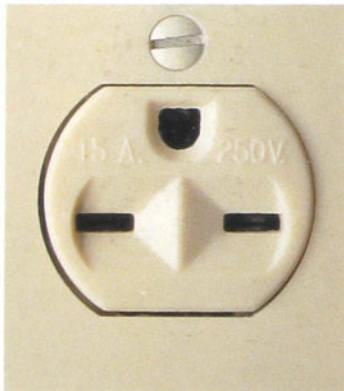
15 amps, 250 volts. This receptacle is used primarily for window air conditioners. It is available as a single unit or as half of a duplex receptacle with the other half wired for 125 volts.
