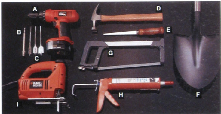
These basic tools are used for advanced wiring projects: drill (A) drill bit extension (B) and spade bits (C) for boring holes in framing members, hammer (D) for attaching electrical boxes, wallboard saw (E) for making cutouts in indoor walls, shovel (F) to dig trenches for outdoor wiring, hacksaw (G) for cutting conduit, caulk gun (H) for sealing gaps in exterior walls, jig saw (I) for making wall cutouts.
