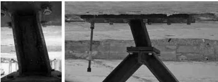
Figure 4.15 Link shear deformation during the test.
