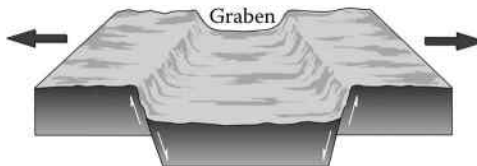
Figure 3.26 Formation of a graben.
