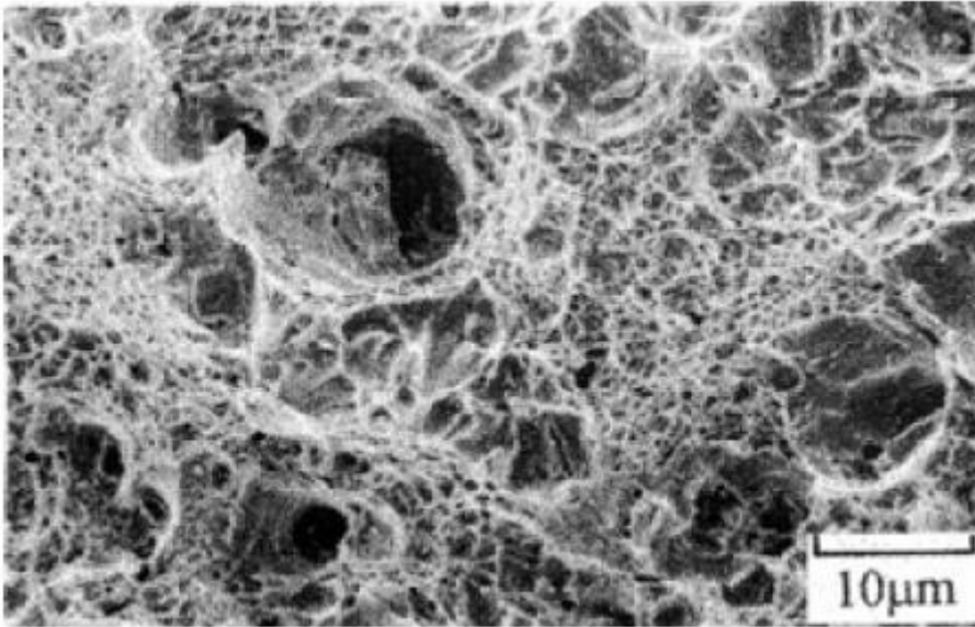
Figure 20. Tensile cavities observed by SEM on fractured surface of tensile tested specimen of B containing modified 304 steel.
