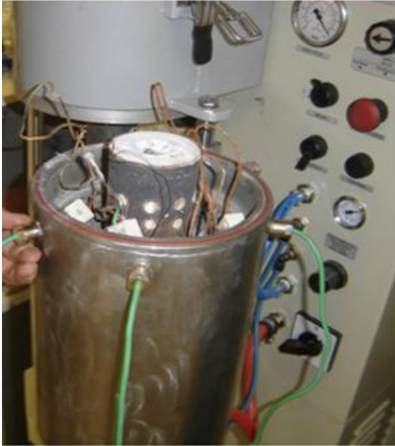
Figure 4. The casting chamber of the vacuum – pressure casting machine with appropriate modifications to accommodate the thermocouples.
