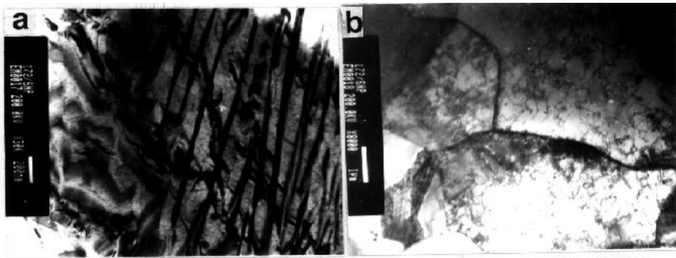
Figure 9. TEM micrographs of steel 1 soaked at 1000°C and deformed 50% at 740°C showing (a) ferrite-pearlite (b) non-polygonal ferrite with higher dislocation density.
