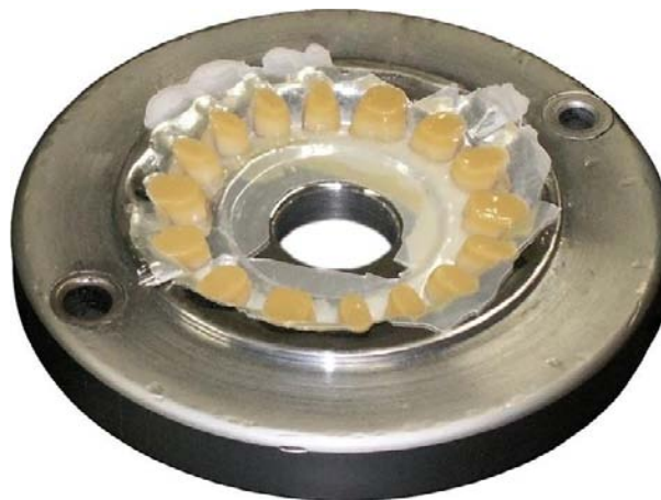
Figure 2. Final mold and molded sets of acrylic teeth with flash.
