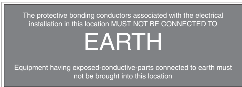
Figure 6.6 Warning notice – protective bonding conductors (reproduced with permission of IET)
