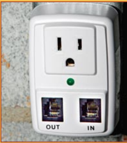
306 | Phone and Coaxial Cable Protection
