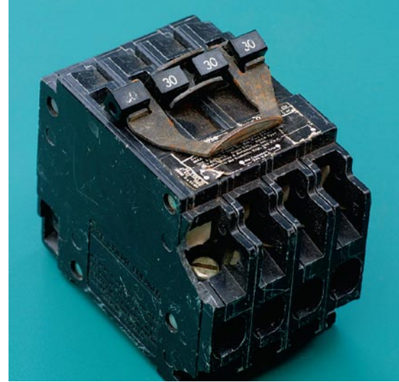
This quad breaker comes as a dual double pole. There is one 30-amp double pole on the two inside terminals. The two outside terminals are ganged together to make a second 30-amp double pole.
