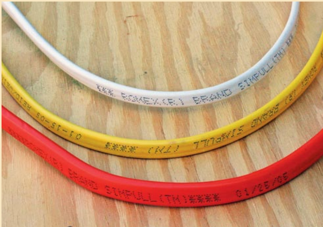
Most cables today use color-coded sheaths to advertise their gauge: white, 14 gauge; yellow, 12 gauge; orange, 10 gauge.
