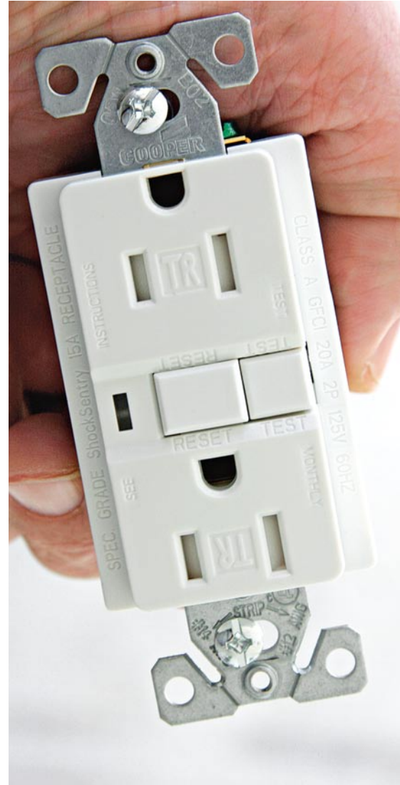
New codes require the use of tamper-resistant receptacles for household 125-volt 15- and 20-amp receptacles. Look for TR on the front.
