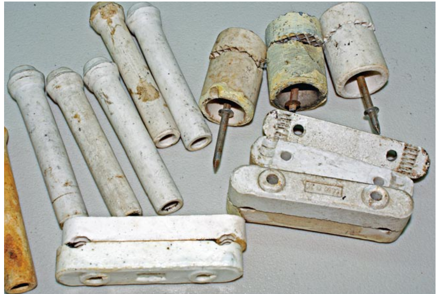
Knob-and-tube wiring got its name from these components. Tubes on the left went through bored holes. Cleats (bottom right) and knobs (top right) held cables on runs along flat sides of joists and walls.
