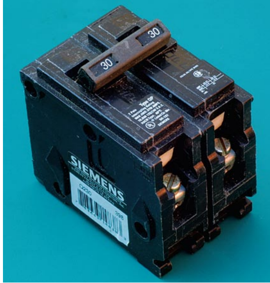
A 2-in.-wide double-pole breaker stabs onto both hot tabs of the panel's bus to power 240-volt and 120/240-volt loads. It consists of two single-pole breakers sharing a common trip.
