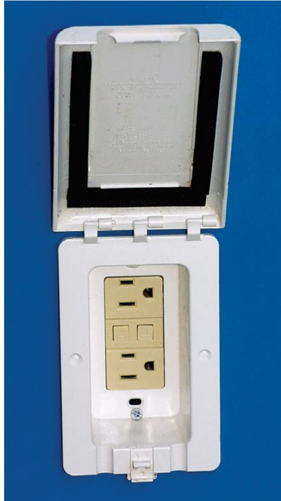
The best performing (and best looking) weatherproof covers are recessed into the wall and have a seal between the flat lid and the box. (See TayMac at www.tay-mac.com .)
