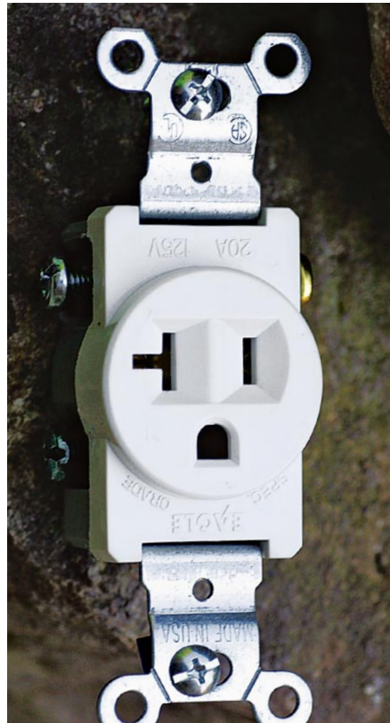
A single receptacle has only one place to plug in a load. Note the horizontal slot, which indicates that it is a 20-amp receptacle and capable of taking cords from heavy-duty, 20-amp appliances.
