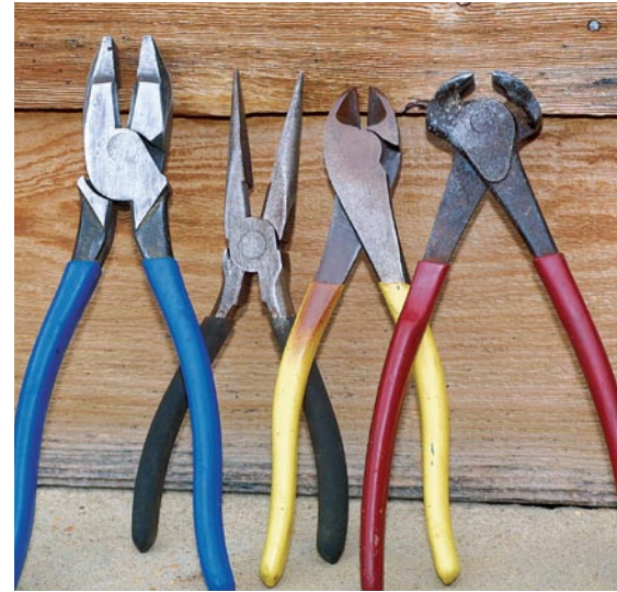
My most-used tools: electrician's pliers (Klein), needle-nose pliers, diagonal cutters (called diagonals), and end cutters (staple pullers). Don't start wiring until you have these tools.
