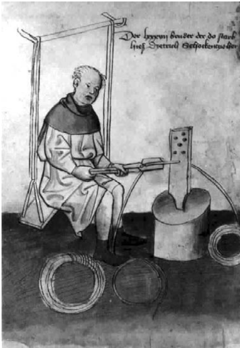
Figure 2.1 Illustration of medieval wire drawing, as presented in the Hausbuch der Mendelschen Zwölfbruderstiftung zu Nürnberg .
