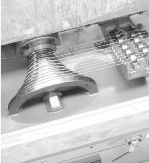
Figure 3.3 A stepped cone within a commercial drawing system. (Courtesy of Machine+Engineering S.r.l.)
