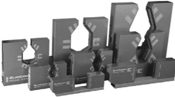
Figure 20.6 ODAC ® heads with calibrated single-scan technology for diameter measurement. (Courtesy of Initial Publications, Inc., Akron, OH, USA).
