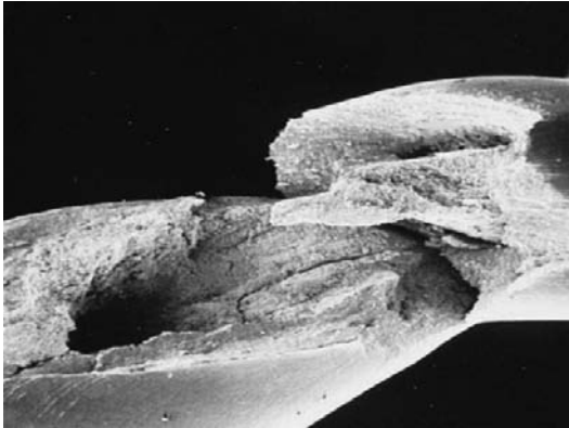
Figure 12.8 Typical example of a wire break due to a center burst. Note “cup” on left, and “core” on right. (Courtesy of Horace Pops)
