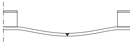
Fig. 16.11 Welding deformations in the transverse splice of the bottom flange plate tend to produce out-of-plane deformations.
