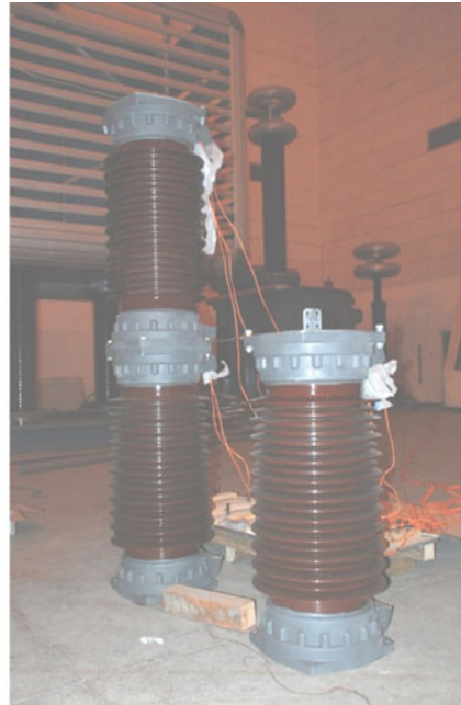
Fig. 11.15 Sketch of the 110 kV thyristor valve controllable arrester’s structure and appearance
