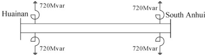
Fig. 12.1 Configuration of HV shunt reactors in Huainan to South Anhui power transmission line
