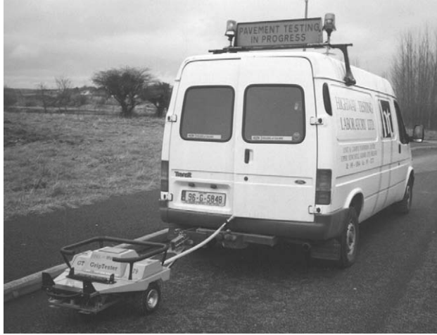
FIGURE 21.4 Griptester in operation.
