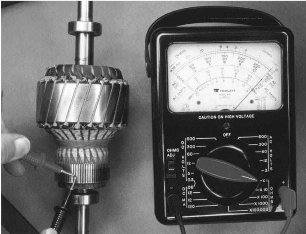
Figure 1-11 Analog ohmmeter being used to measure armature resistance.
