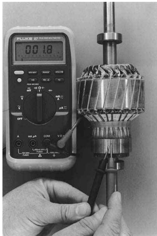
Figure 1-13 Digital ohmmeter being used to measure resistance.
