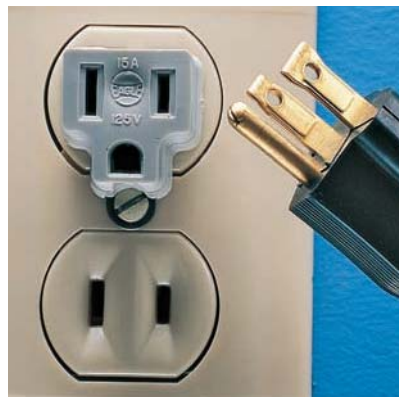
A receptacle adapter allows three-prong plugs to be inserted into two-slot receptacles. The adapter should only be used with receptacles mounted in a bonded metal box, and the grounding loop or wire of the adapter must be attached to the coverplate mounting screw.
