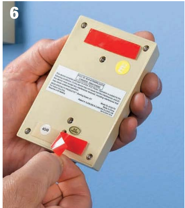
6 Remove the backing from the adhesive pads on the back of the wireless switch transmitter box. Install a new 9-volt battery (or other type as required) in the box, and connect it to the switch transmitter terminals.
