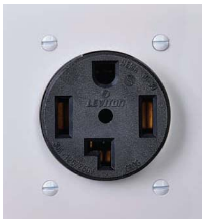
30 amps, 120/240 volts. This grounded receptacle is used for clothes dryers. It provides high-voltage current for heating coils and 120-volts to run lights and timers.
