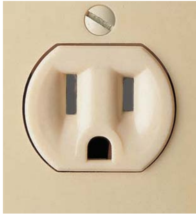
15 amps, 120 volts. Three-slot grounded receptacles have two different-sized slots and a U-shaped hole for grounding which is required in all new wiring installations.
