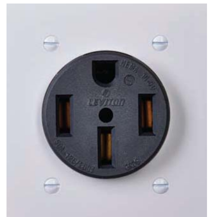
50 amps, 120/240 volts. This new, grounded receptacle is used for ranges. The high voltage powers heating coils, and the 120-volts run clocks and lights.
