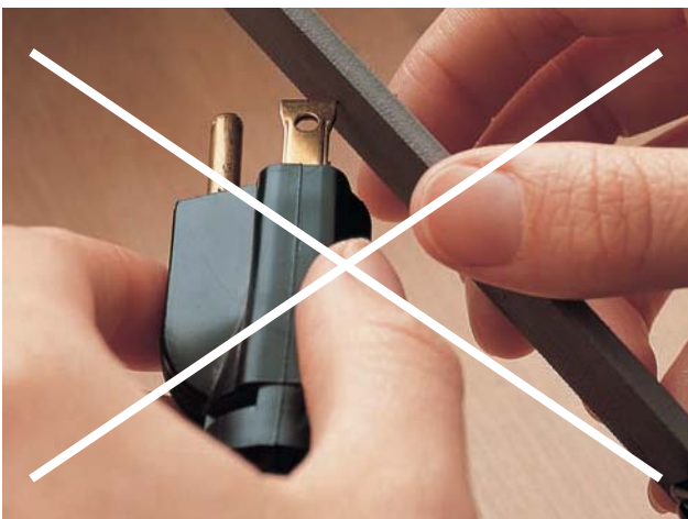
Never alter the prongs of a plug to fit a receptacle. If possible, install a new grounded receptacle.
