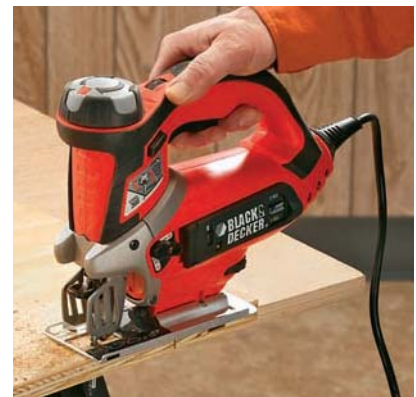
Double-insulated tools have non-conductive plastic bodies to prevent shocks caused by ground faults. Because of these features, double-insulated tools can be used safely with ungrounded receptacles.
