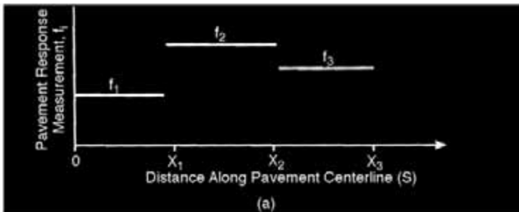
FIGURE 66.3 Pavement segment delineation with the response-based approach.
