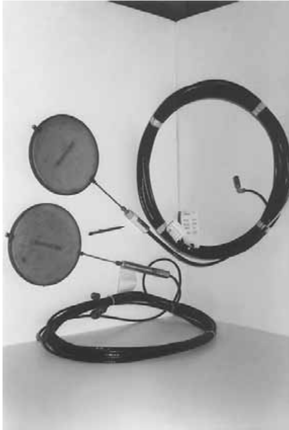
FIGURE 28.5 Pressure cells for measurement of stresses in soil masses or contact stresses between soil masses and concrete or steel surfaces. (Picture courtesy of A. Bernal and A. Karim, Bechtel Geotechnical Laboratory, Purdue University.)
