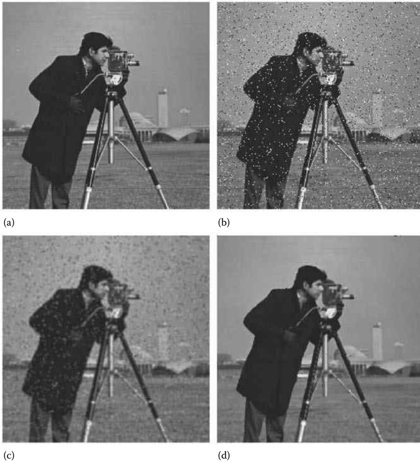
FIGURE 26.1 The original figure depicted in (a) is corrupted with transmission noise, the result of which is given in (b). The received image is then processed with (c) linear (mean) and (d) nonlinear (median) filters.
