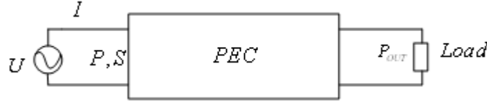
Figure 1. Powers in conversion of AC electrical energy
