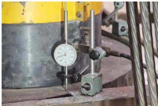
Figure 13.14 Dial gauge measurement of pile head settlement.
