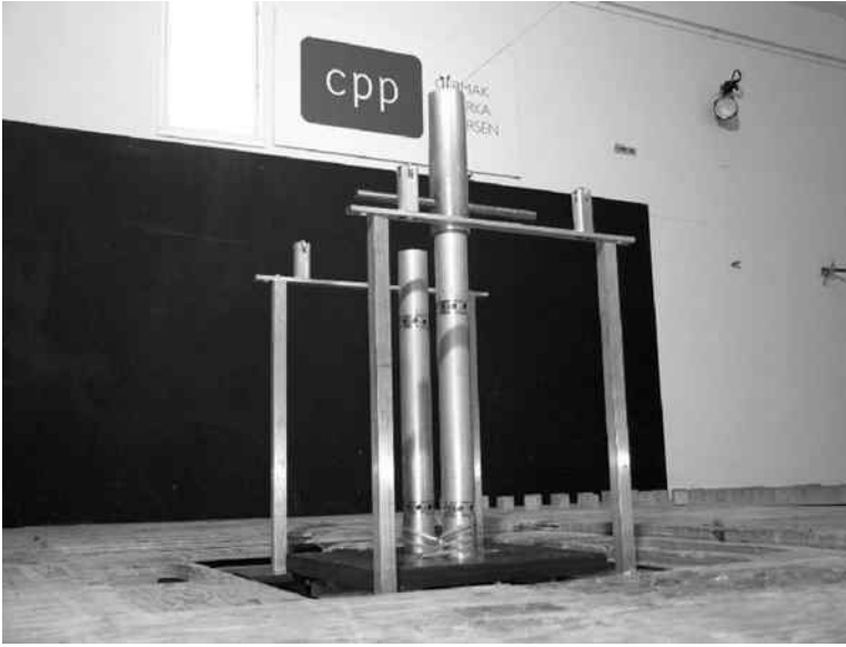
FIGURE 4.3 Rigid AM mounted as a flexible steel bar.
