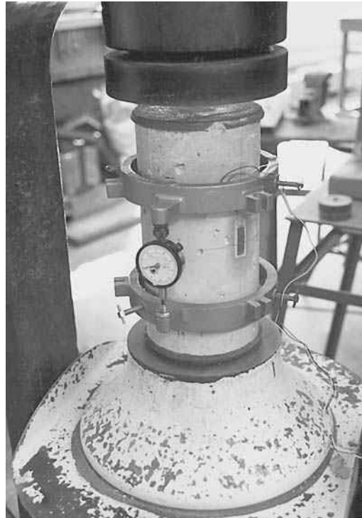
Test on a standard concrete cylinder to determine the modulus of elasticity of concrete.
