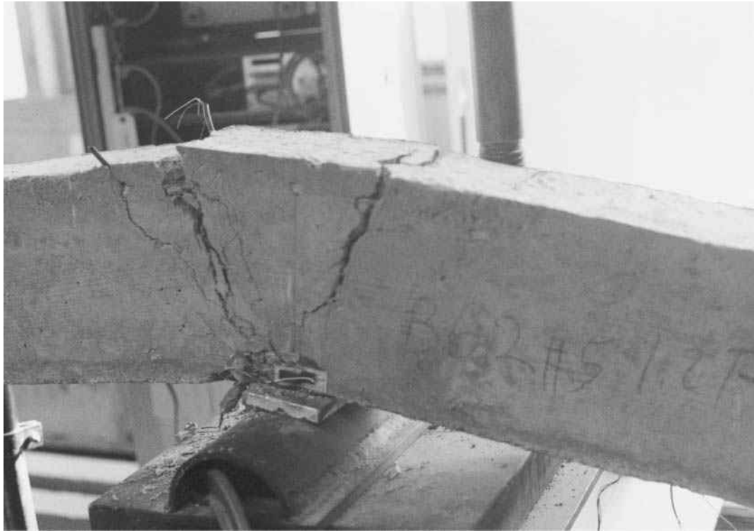
Plastic hinge in the maximum negative moment region.
