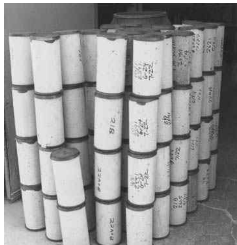
Standard capped cylinders ready for testing.
