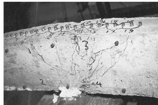
Failure conditions at the positive- and negative-moment sections in a continuous reinforced concrete beam.
