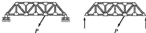
**FIG. 3.11** An Example of Externally Statically Unstable Plane Structure
