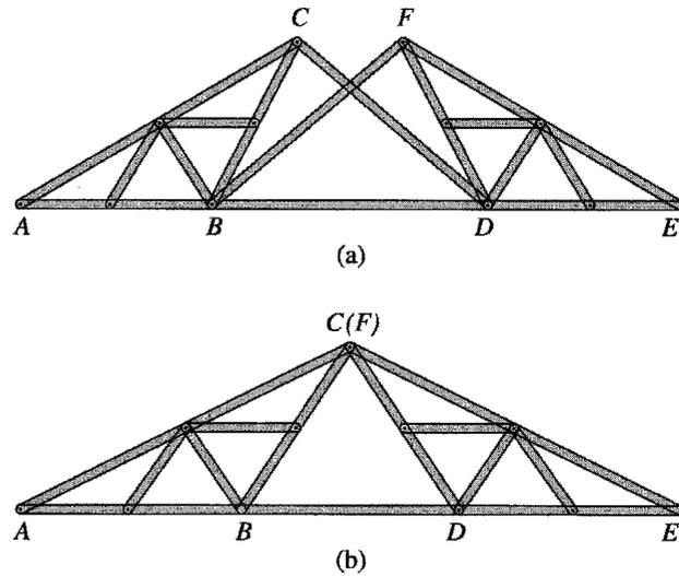
FIG. 4.11 Compound Trusses
