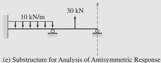
(e) Substructure for Analysis of Antisymmetric Response
