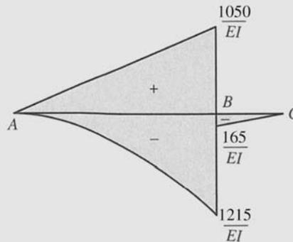
(b)  $\frac{M}{EI}$  Diagram ( $\frac{\text{kN-m}}{EI}$ )
