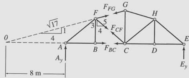
(g) Section *aa*
