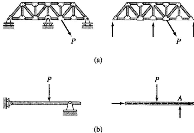
**FIG. 3.12** Reaction Arrangements Causing External Geometric Instability in Plane Structures
