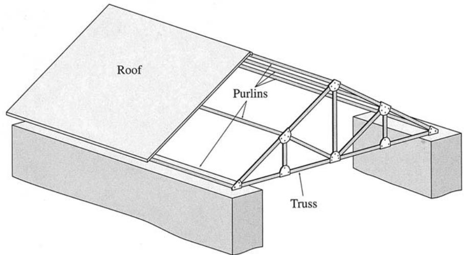
**FIG. 4.3** Framing of a Roof Supported by Trusses
