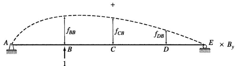
(c) Primary Beam Loaded with Redundant  $B_y$
