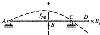
(c) Primary Beam Loaded with Redundant  $B_y$
