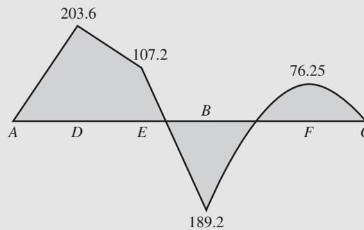
Bending moment diagram (kN-m)
