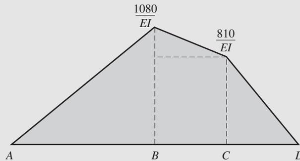
(b)  $\frac{M}{EI}$  Diagram ( $\frac{\text{kN-m}}{EI}$ )
