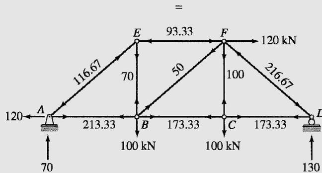
(b) Primary Truss Subjected to External Loads— $F_O$  Forces
