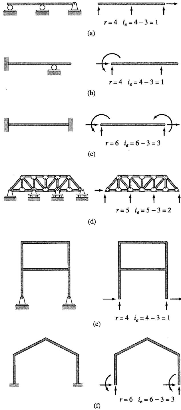
**FIG. 3.10** Examples of Externally Statically Indeterminate Plane Structures
