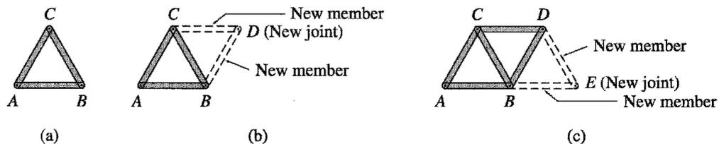
FIG. 4.10 Simple Truss
