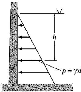
FIG. 2.9 Hydrostatic Pressure
