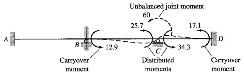
(d) Balancing Joint  $C$
