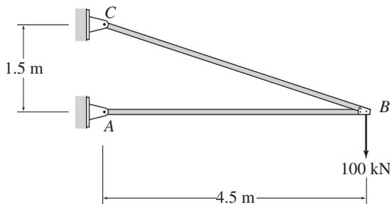
$$\begin{aligned} EA &= \text{constant} \\ E &= 70 \text{ GPa} \\ A &= 4000 \text{ mm}^2 \end{aligned}$$
