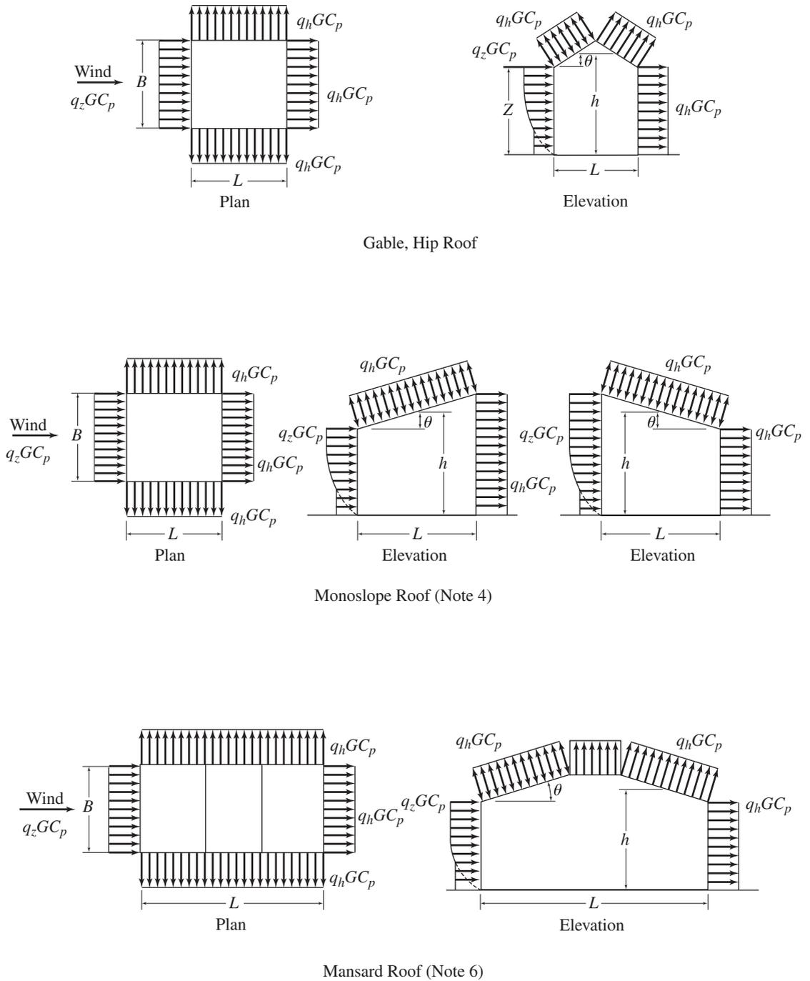
**FIG. 2.5** External Pressure Coefficients,  $C_p$ , for Loads on Main Wind-Force Resisting Systems for Enclosed or Partially Enclosed Buildings of All Heights
