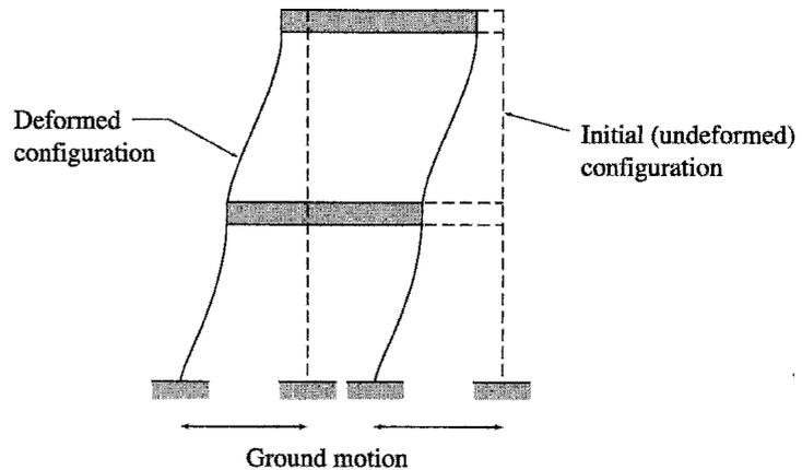
FIG. 2.8 Effect of Earthquake on a Structure
