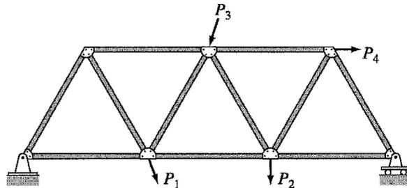
FIG. 1.8 Plane Truss
