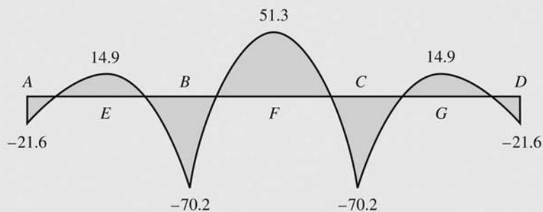
(f) Bending Moment Diagram (kN-m)
