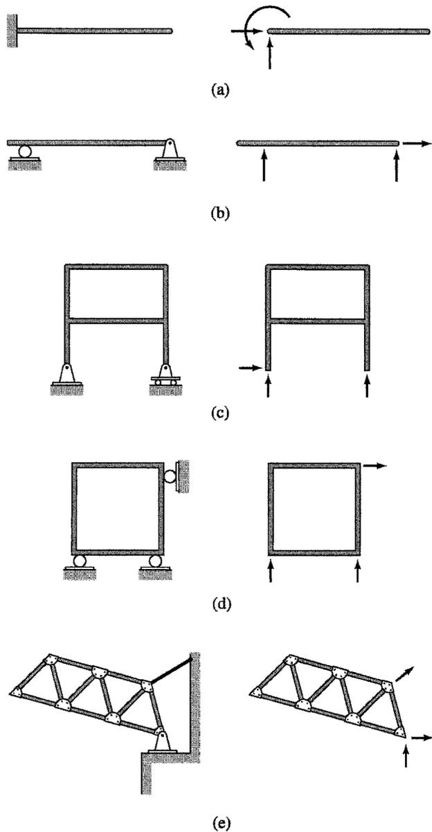
**FIG. 3.9** Examples of Externally Statically Determinate Plane Structures
