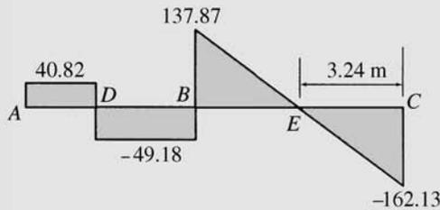
(e) Shear Diagram (kN)
