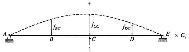
(d) Primary Beam Loaded with Redundant  $C_y$
