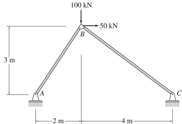
$$\begin{aligned} EA &= \text{constant} \\ E &= 70 \text{ GPa} \\ A &= 1,000 \text{ mm}^2 \end{aligned}$$
