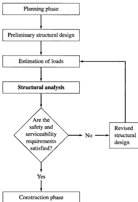
**FIG. 1.2** Phases of a Typical Structural Engineering Project
