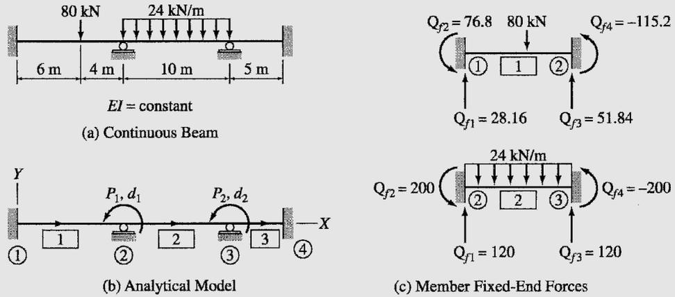
$$S = EI \begin{bmatrix} 1 & 2 \\ (0.4 + 0.4) & 0.2 \\ 0.2 & (0.4 + 0.8) \end{bmatrix} \begin{matrix} 1 \\ 2 \end{matrix} = EI \begin{bmatrix} 1 & 2 \\ 0.8 & 0.2 \\ 0.2 & 1.2 \end{bmatrix} \begin{matrix} 1 \\ 2 \end{matrix}$$
