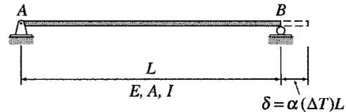
(a) Statically Determinate Beam
