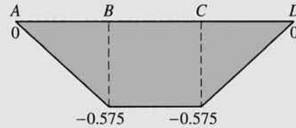
(f) Influence Line for  $F_{BC}$  (kN/kN)
