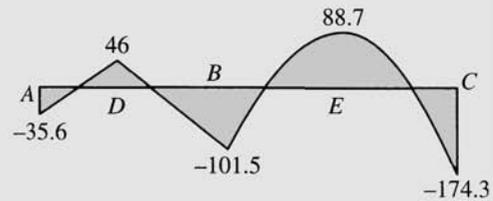
(f) Bending Moment Diagram (kN-m)
