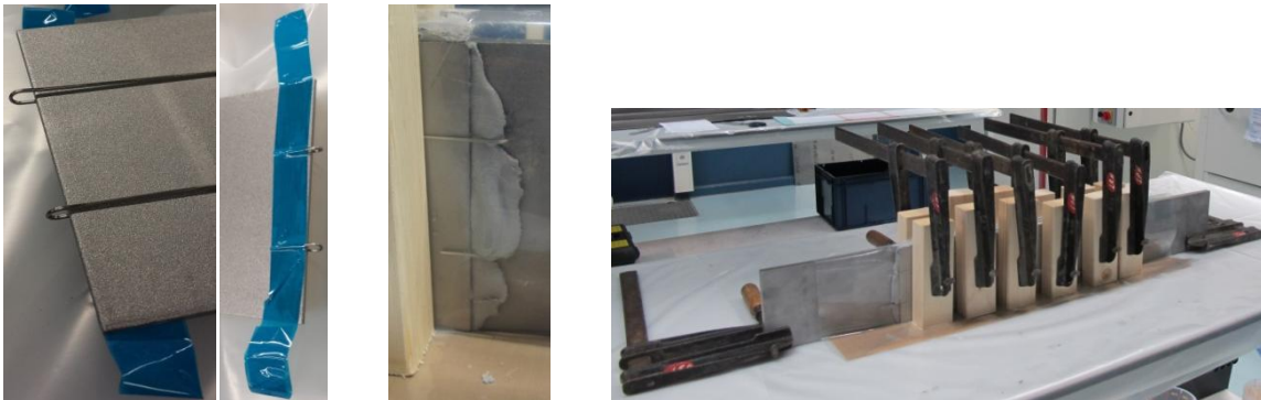
Figure 13.10: Pictures of the bonding of the straps to the plates; application of spacer with tape, outflow of the adhesive after tightening the clamps and connection during hardening
