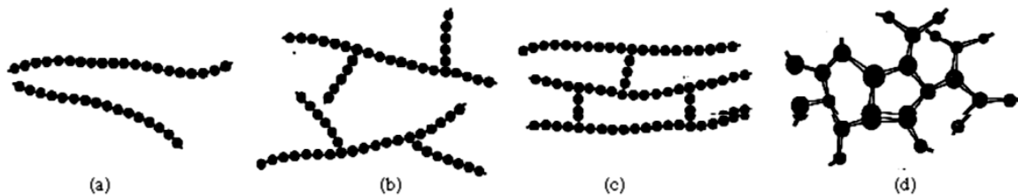
Figure 4.1: Schematic illustration of a linear, (b) branched, (c) cross-linked and (d) network (3D) molecular structures [10]
