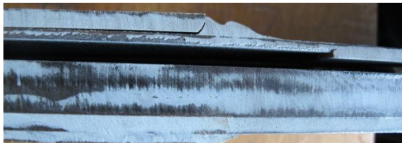
Figure 31.65: Connection 5 – direction y- – end of second lap
