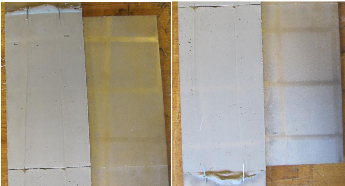
Figure 31.5: Connection 1 – side 1 – direction z+ (left side) and direction z- (right side) – first adhesive layer – complete delamination caused by adhesion failure
