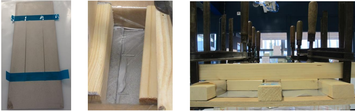
Figure 13.7: Pictures of the manufacturing of the straps; application of spacer with tape, outflow of the adhesive after tightening the clamps and mould with straps during hardening
