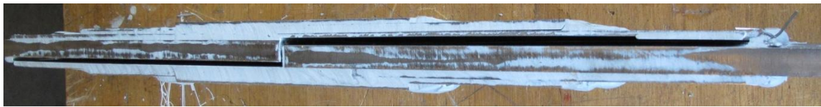
Figure 31.60: Connection 5 – Failure in Z-shape
