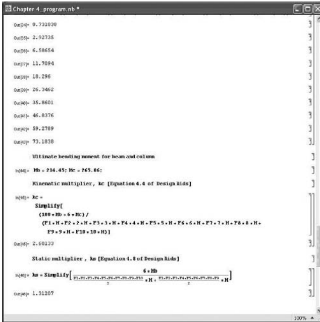
IMAGE 6.6 Five bay-ten story regular frame; coding in Mathematica_page 5.
