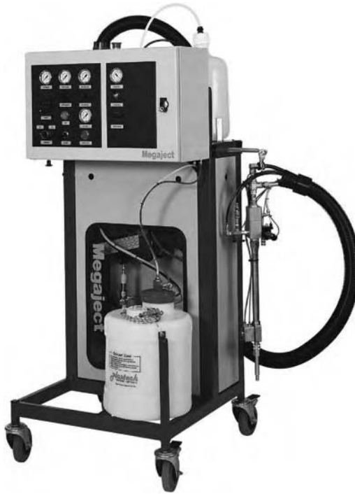
FIGURE 3.8 RTM equipment used at the CFC, West Virginia University.
