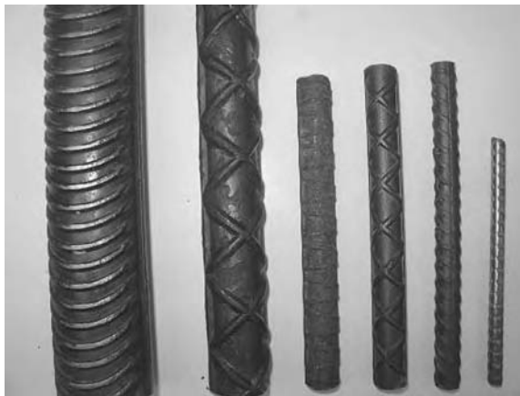
FIGURE 2.6 Examples of deformed bars with varying lug (rib) configurations.
