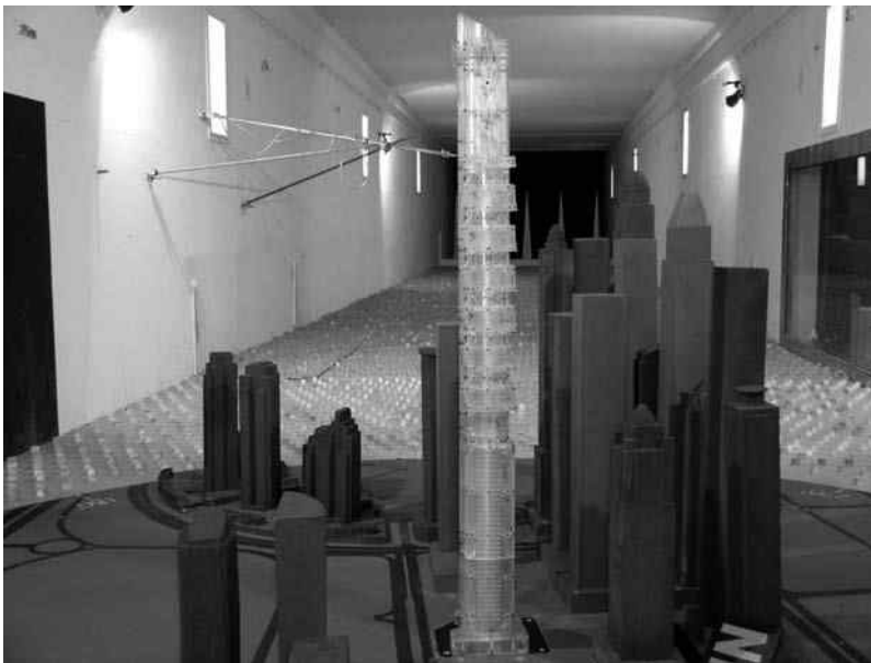
FIGURE 4.38 Close-up of model in wind tunnel: Pentominium, Dubai. (Courtesy of CPP Wind Engineering & Air Quality Consultants.)
