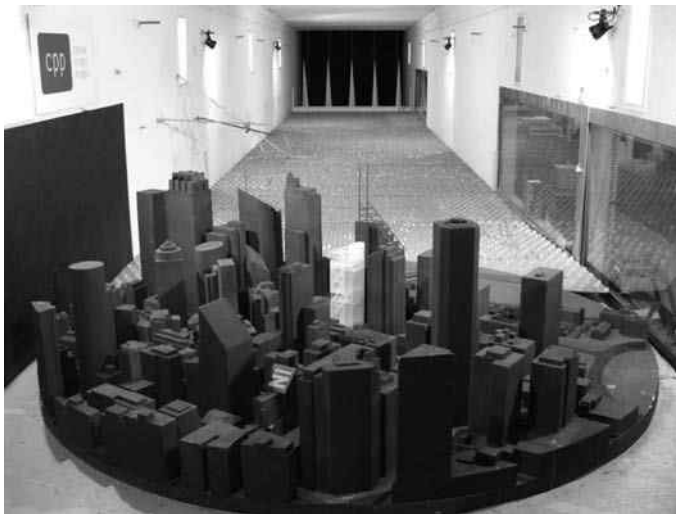
FIGURE 4.36 Photographs of rigid model in wind tunnel. Chifley Plaza, Sydney. (Courtesy of CPP Wind Engineering & Air Quality Consultants.)
