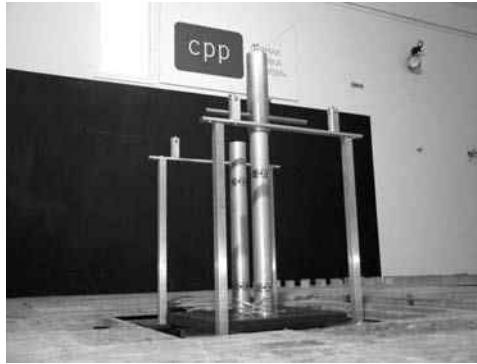
FIGURE 4.43 Rigid aeroelastic model mounted on a flexible steel bar.
