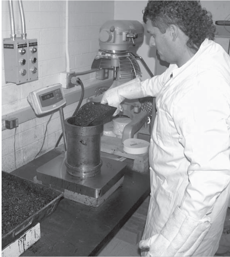
FIGURE A.57 Placing HMA in mold.
