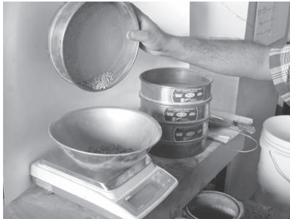
FIGURE A.23 Weighing aggregate retained in sieves.
