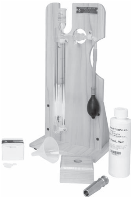
FIGURE 6.3 Blaine air permeability apparatus. (Courtesy of Humboldt Mfg. Co.)
