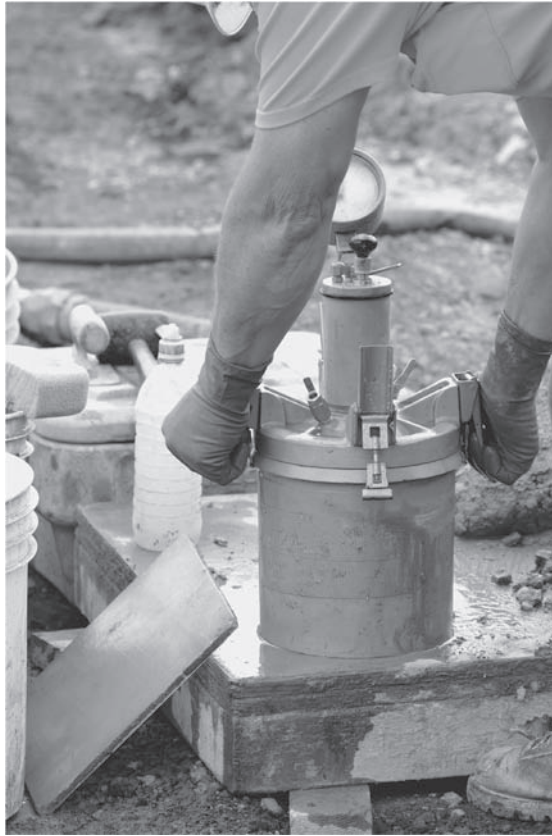
FIGURE A.34 Reading pressure meter. (Shutterstock/TFoxFoto)
