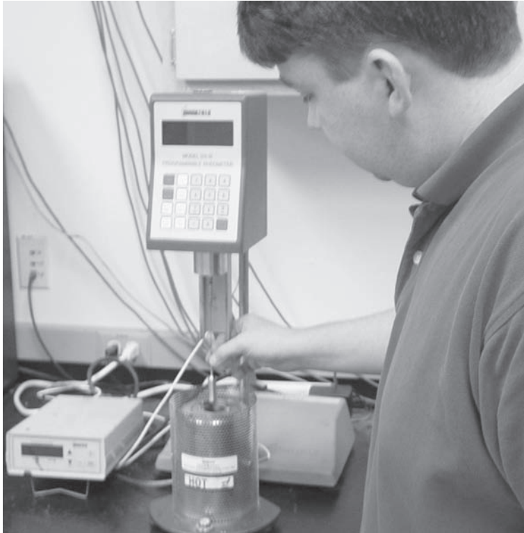
FIGURE A.52 Inserting the spindle into chamber for the rotational viscometer test.
