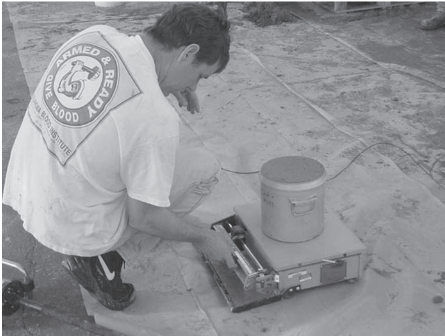
FIGURE A.33 Weighing concrete inside the container.
