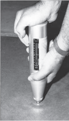
FIGURE 7.39 Rebound hammer for nondestructive evaluation of hardened concrete.
