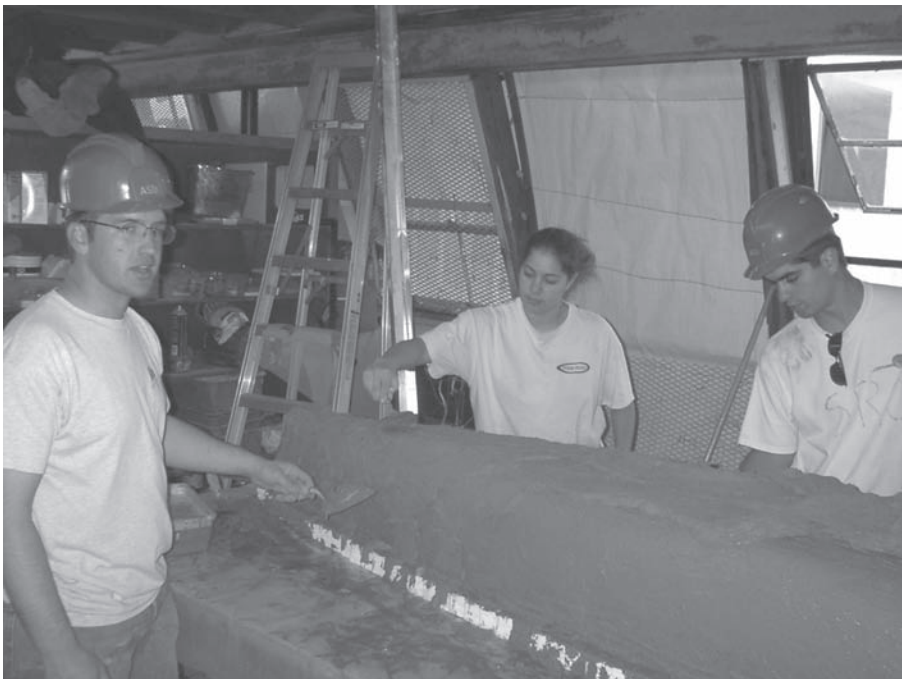
FIGURE 7.49 ASCE students at Arizona State University making a concrete canoe using lightweight concrete.
