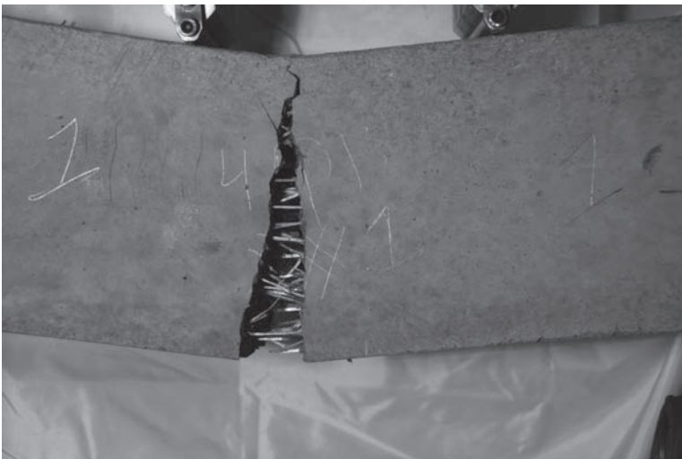
FIGURE 11.19 Fiber bridging cracks in concrete. (Courtesy of Barzin Mobasher)
