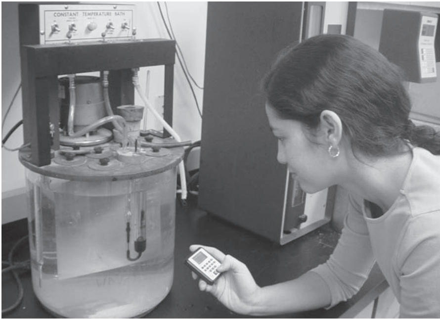
FIGURE A.56 Measuring flow time using a stop watch.
