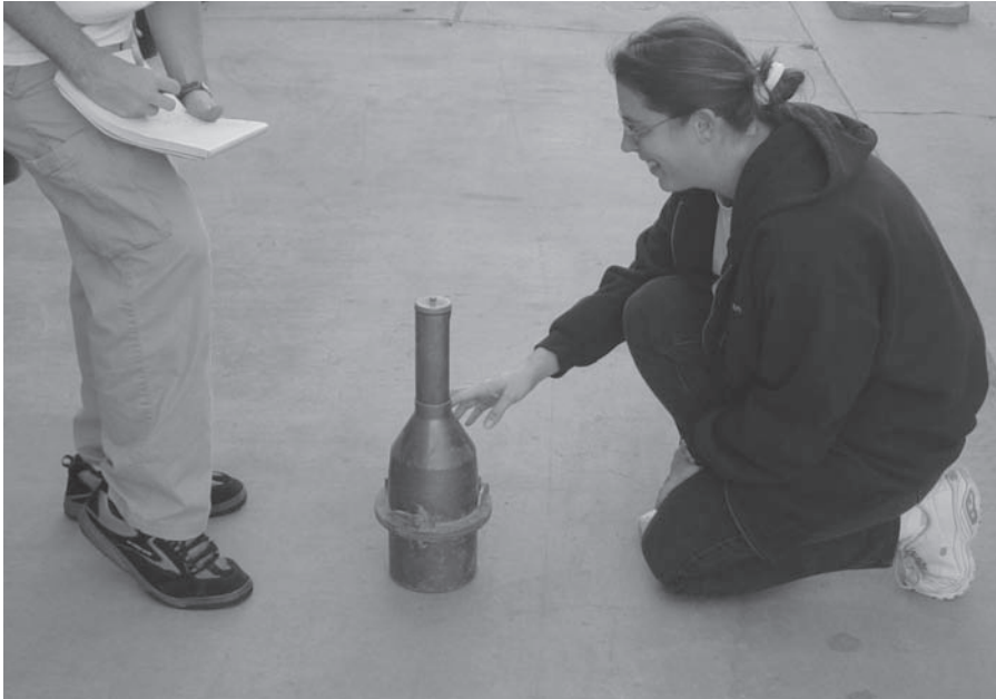
FIGURE A.35 Reading air meter.
