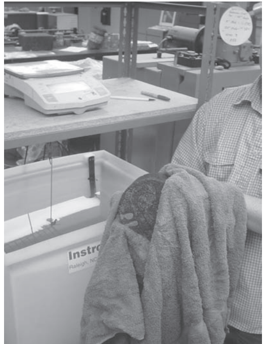
FIGURE A.65 Weighing HMA specimen in water.
