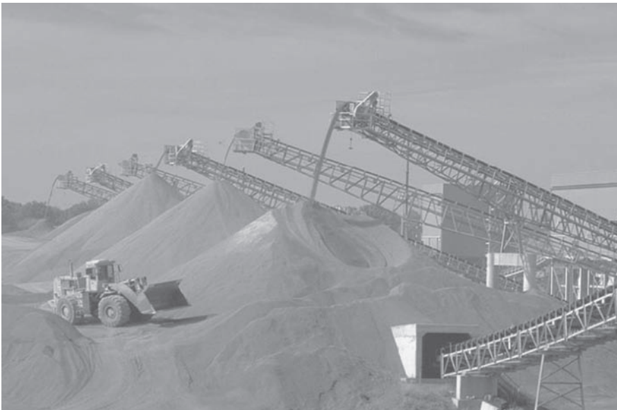
FIGURE 5.1 Aggregate stockpiling. (Courtesy of FHWA)
