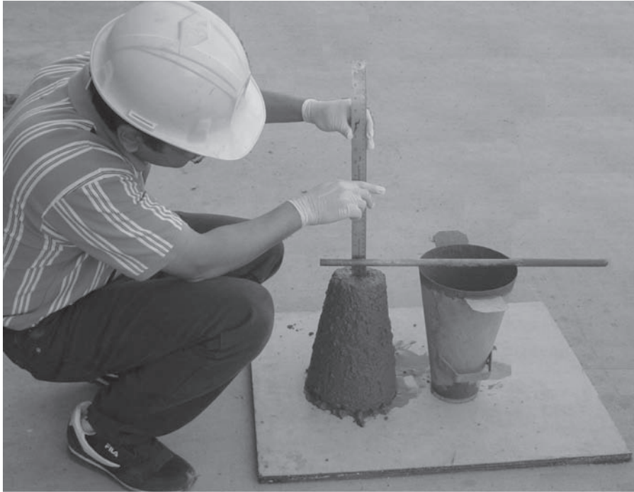
FIGURE A.32 Measuring the slump of freshly mixed concrete.
