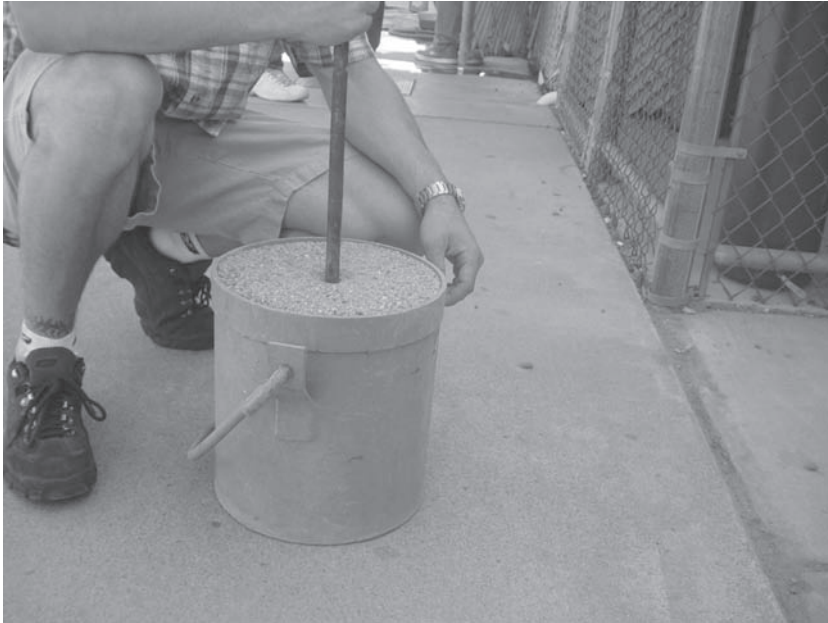
FIGURE A.28 Rodding aggregate in the container.
