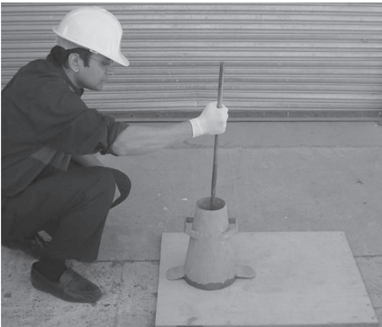
FIGURE A.31 Rodding fresh concrete in the slump cone with a tamping rod.
