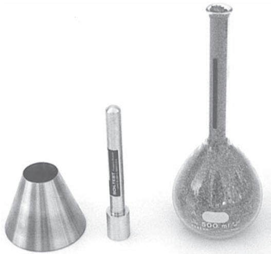
FIGURE A.27 Mold, tamper, and volumetric flask used to determine bulk specific gravity and absorption of fine aggregate.
