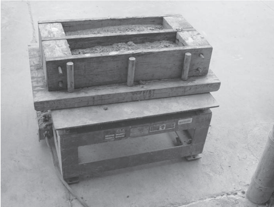
FIGURE A.38 Consolidating concrete in a beam mold using an external vibrator.
