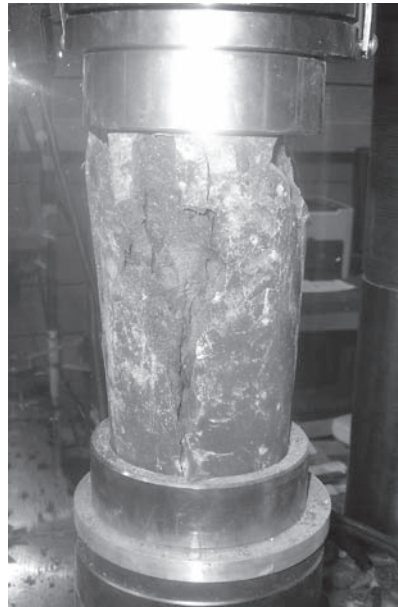
FIGURE A.44 Example of fracture with vertical cracks. (Courtesy of FHWA)
