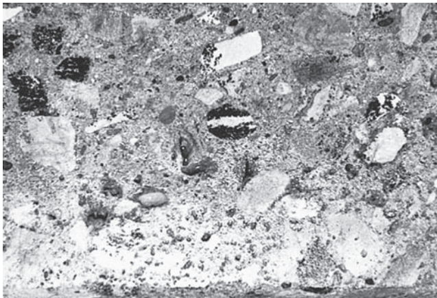
FIGURE 11.15 Cross section of portland cement concrete showing cement paste and aggregate particles.
