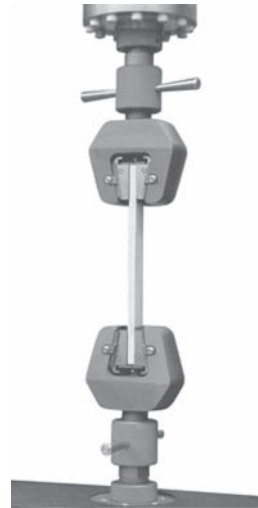
FIGURE A.75 Tension test on an FRP composite specimen. (Courtesy of Intertek Plastics Technology Laboratories)
