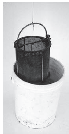
FIGURE A.26 Wire basket and water tank used to determine bulk specific gravity and absorption of coarse aggregate.
