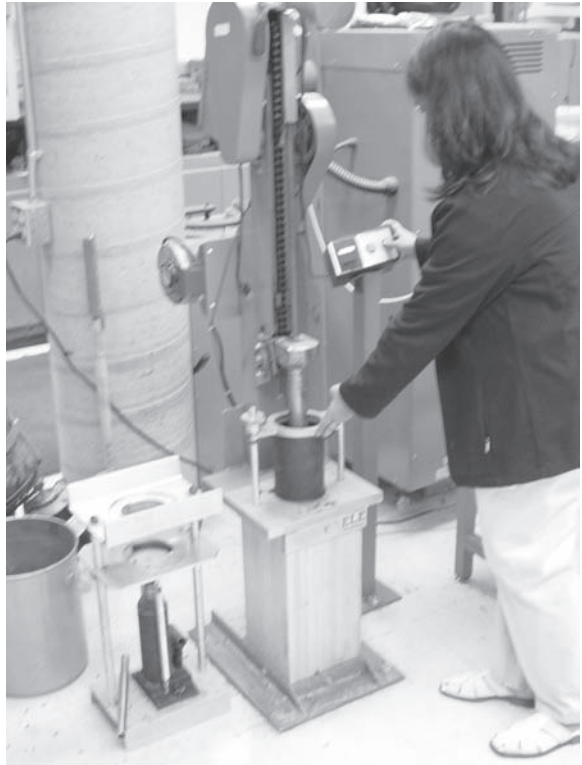
FIGURE A.62 Compacting an HMA specimen using a mechanical Marshall hammer.
