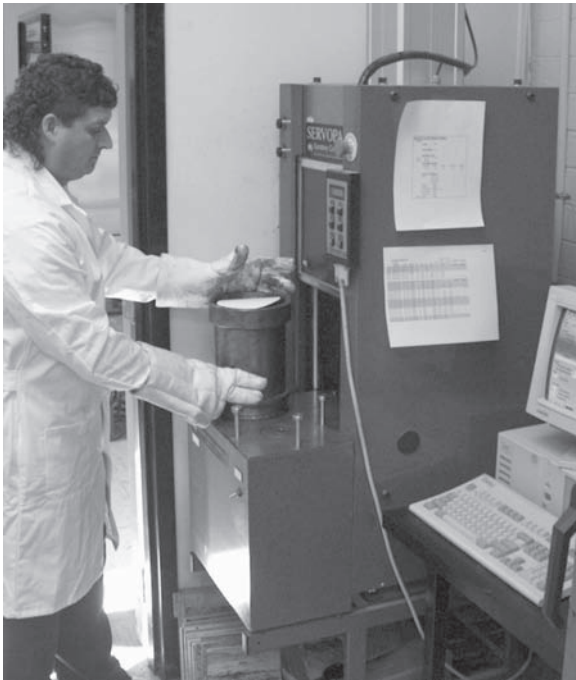
FIGURE A.58 Placing the mold in the gyratory compactor.
