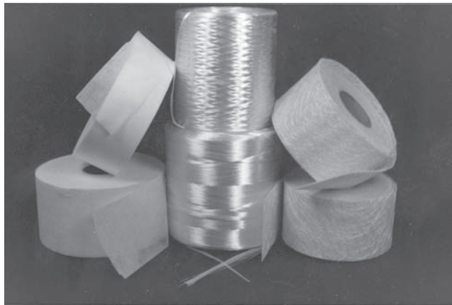
FIGURE 11.4 Common continuous glass fibers (veil, roving, and mat). (Courtesy of Creative Pultrusions, Inc.)
