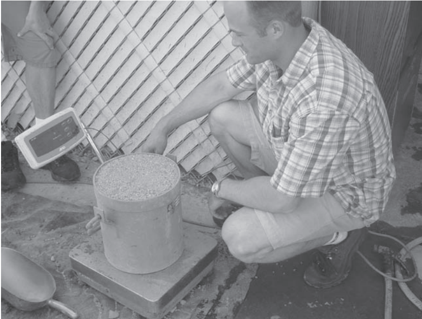
FIGURE A.29 Weighing the aggregate.
