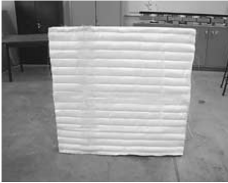
FIGURE 9.34 Sandwich composite panel with StructoGard fire insulation before the UL 1709 fire exposure test.
