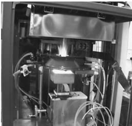
FIGURE 9.12 Cone calorimeter (ASTM E 1354) heat release test.
