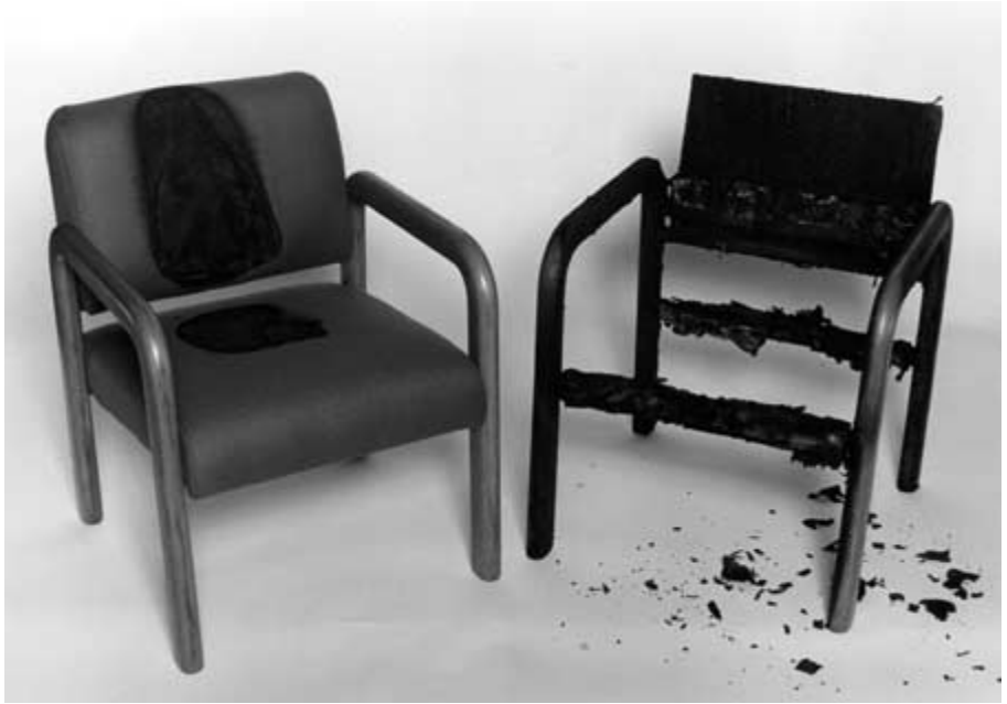
FIGURE 5.19 Chairs tested using CAL 133 protocol, showing the impact of a fire blocking interliner.
