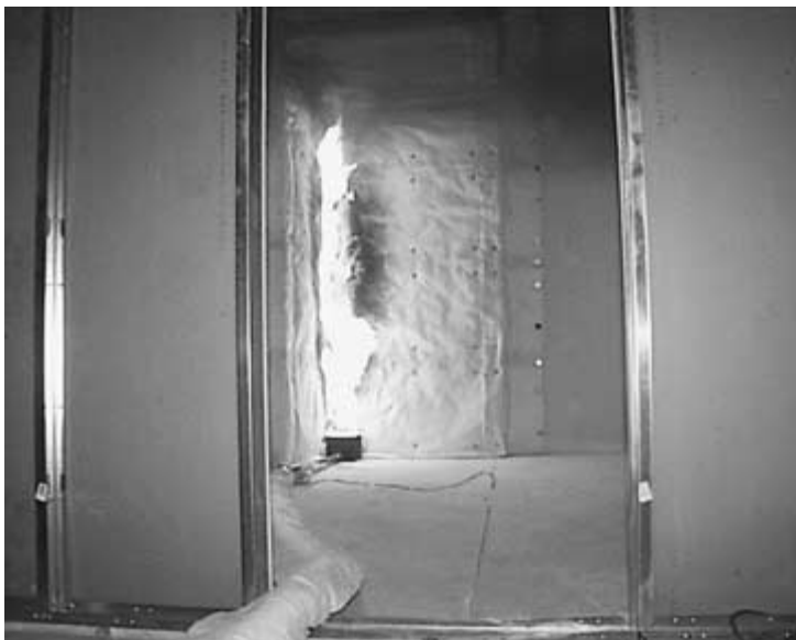
FIGURE 9.16 ISO 9705 fire test during 100-kW fire exposure.
