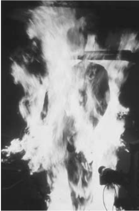
FIGURE 5.5 Flash fire exposure using instrumented thermal mannequin.
