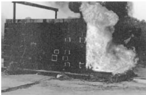
FIGURE 9.26 Postflashover fire in the U.S. module, west end, near the end of the test.
