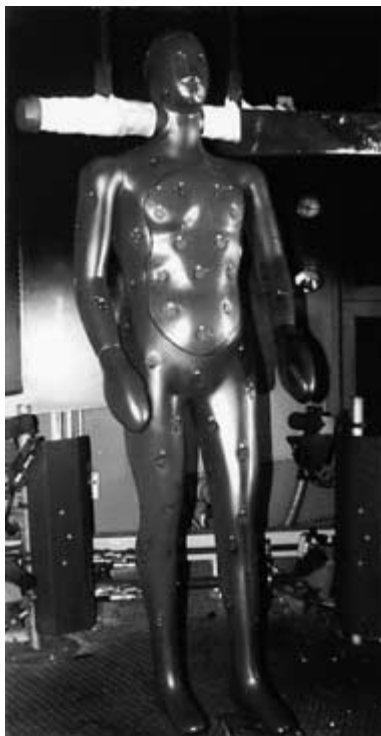
FIGURE 5.4 Instrumented thermal mannequin apparatus.
