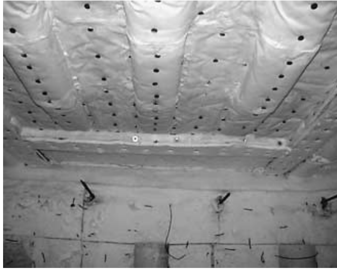
FIGURE 9.31 Solid composite deck panel with fire insulation (Test 4) in the furnace before the fire test.
