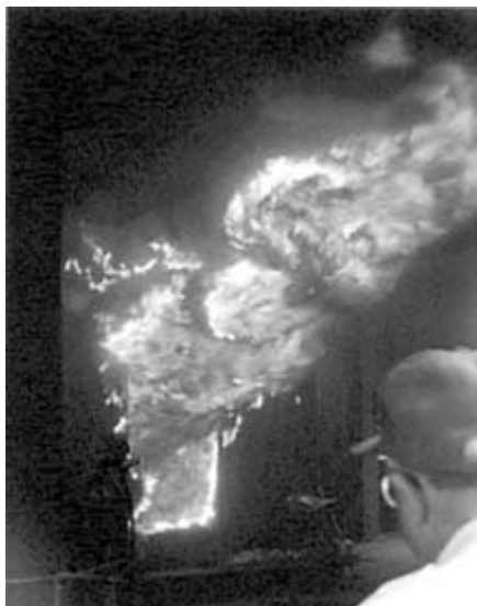
FIGURE 9.26 Postflashover fire in the U.S. module, west end, near the end of the test.
