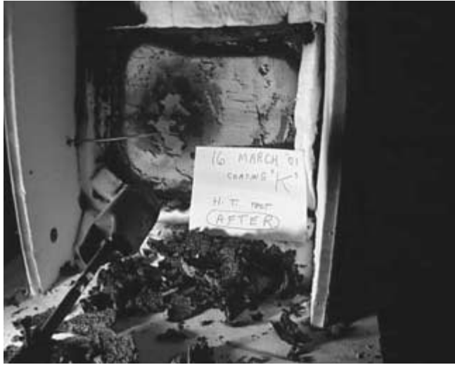
FIGURE 9.58 Coating K in the simulated UL 1709 with char pieces that fell off.
