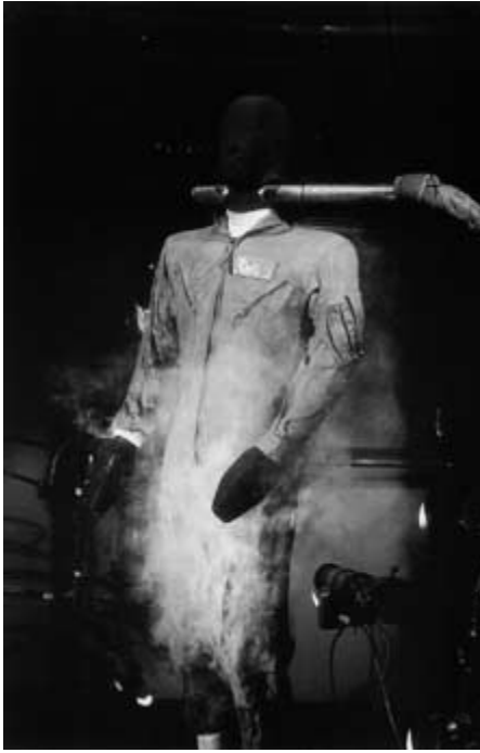
FIGURE 5.7 Nomex® coverall self-extinguishes after torches extinguish.
