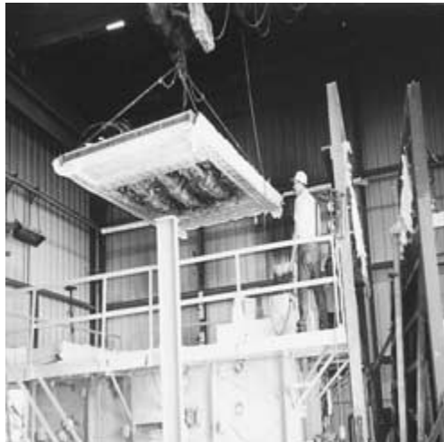
FIGURE 9.32 Solid composite deck panel after the UL-1709 fire resistance test (Test 4).
