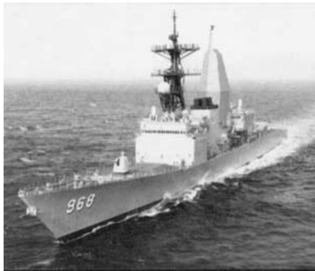
FIGURE 9.3 Composite mast installed aboard USS Radford (DD968). (From Ref. 3)
