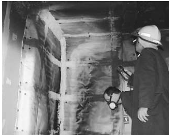
FIGURE 9.20 Composite corner with StructoGard after testing.
