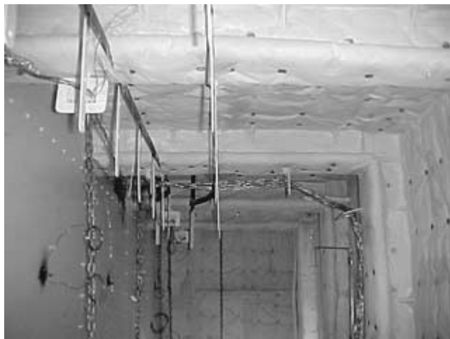
FIGURE 9.60 View of test bulkhead and insulated, non-test surfaces.
