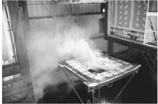
FIGURE 9.35 Sandwich composite panel with StructoGard fire insulation after the UL 1709 fire exposure test.
