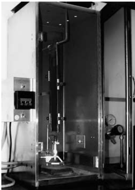
FIGURE 5.1 Vertical flammability test apparatus.
