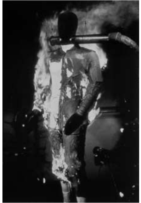
FIGURE 5.6 Flammable coverall continues burning after torches extinguish.
