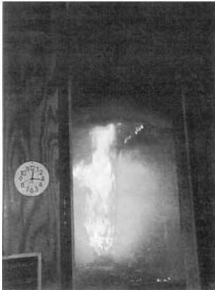
FIGURE 9.17 Material No. 5 just prior to flashover.
