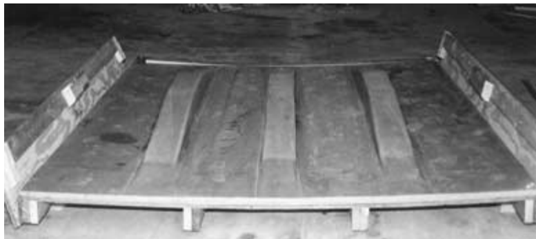
FIGURE 9.30 Solid composite deck panel (Test 4) before the fire insulation.
