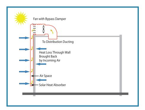
**Figure 5.12**Solar ventilation air preheating is a solar technology that is simple and cost effective.
