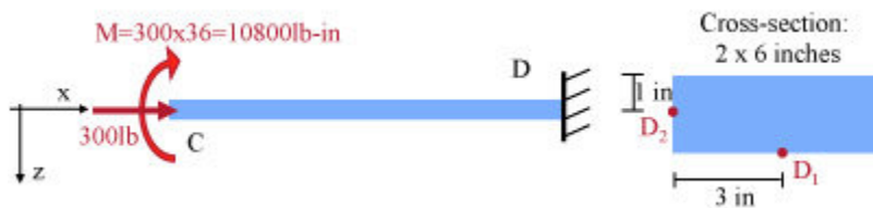
Figure M-10 The beam in Figure M-9 can be reduced to the one shown here by moving the applied force at C, as typically done in statics.
