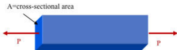
Figure D-12 A bar of cross sectional area A loaded by load P .
