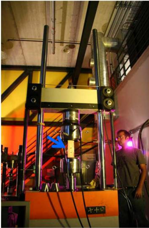
Figure D-1 A mechanical testing machine. The arrow points to the sample being tested.
