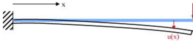
Figure N-1 A beam deflects under external load. At location x , the deflection is u(x) .
