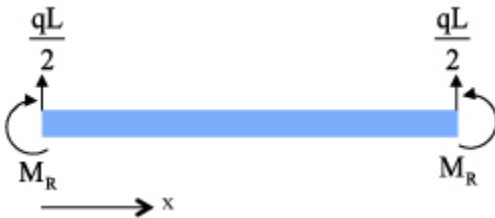
Figure N-21 The free body diagram of the beam in Figure N-20
