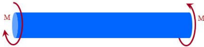
Figure A-4 A torsional shaft.
