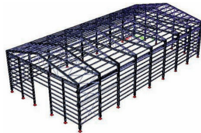
Fig. 2.1. Model for a single story industrial building
