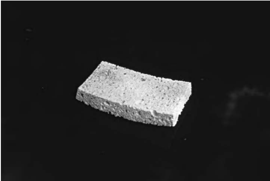
Figure 14.1 A kitchen sponge curls as it dries. So does a floor slab
