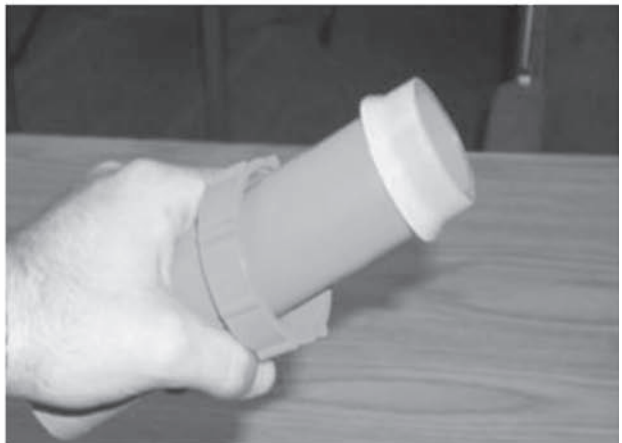
Tighten nut one quarter-turn past hand-tight using a plastic spanner wrench.
