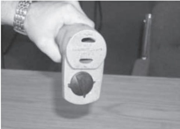
After cutting and deburring pipe, use pipe tool to groove pipe.
