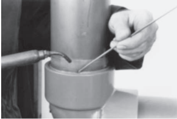
Using an appropriate hot-air welding gun and maintaining uniform heat and pressure on the rod, weld a root bead into the prepared joint area.
