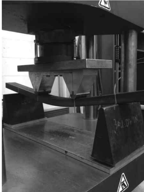
FIGURE 9–1 (See color insert.) Beam deflection is a critical consideration in the performance of many products and structures. Laboratory testing like the four-point loading arrangement shown here can enhance our understanding of this phenomenon.
