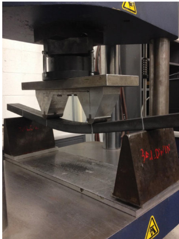
FIGURE 9-1 Beam deflection is a critical consideration in the performance of many products and structures. Laboratory testing like the four-point loading arrangement shown here can enhance our understanding of this phenomenon.
