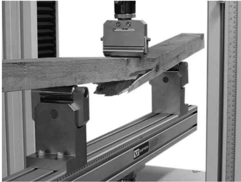
FIGURE 8-1 (See color insert.) Wood beams are particularly susceptible to failure not due to bending stresses as calculated in the last chapter, but instead due to failure in shear. In many applications, designers must take care to analyze shear stress to avoid failures like the one shown in this test fixture.
