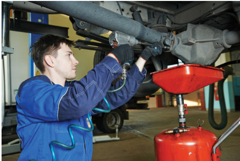
FIGURE 4-1 We depend every day on elements that are loaded in torsion. In this illustration, the driveshaft over the mechanic's head transmits torque generated by the engine to the wheels of the vehicle. Also, since the mechanic is holding a torque gun in his right hand to tighten and loosen fasteners, the relatively small shaft that he holds with his left hand is loaded in torsion as well. Designers are responsible for limiting the amount of stress and deformation in these types of components.
