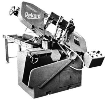
Figure 10.2 Band saw in resting position Type LBU 421 (photo by A. Mössmer, Mutlangen)
