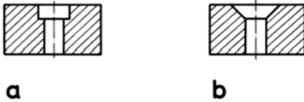
Figure 9.3 Stepped holes a created with counterbore (cylindrical tool), b created with countersink (conical tool)
