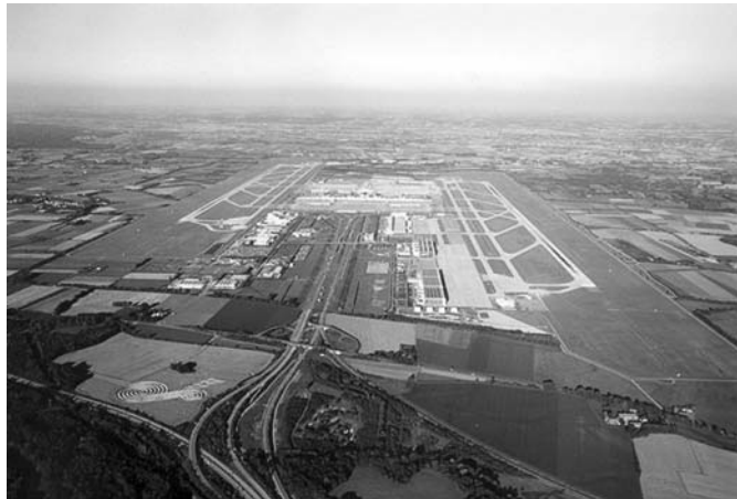
Figure 13.15(b) Landside spinal access layout showing highway link on left and rail link on the right. (Courtesy of Munich Airport.)
