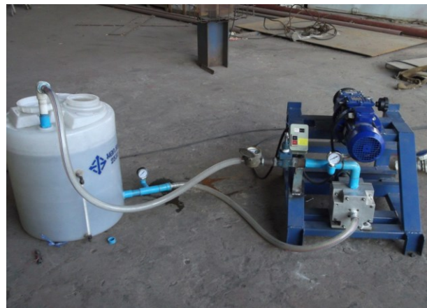
Fig. 4: Testing equipment for scroll pump
