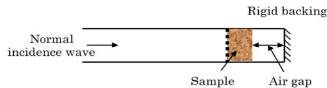
Fig. 5 Sketch of the palm date fibers sample and the PP inside the impedance tube
