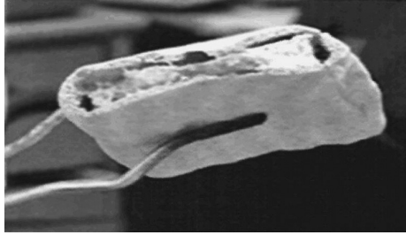
FIGURE 8.6 Cross-section of the EFPS sample after the fire test. One can see a molten sample within the rigid shell casing.
