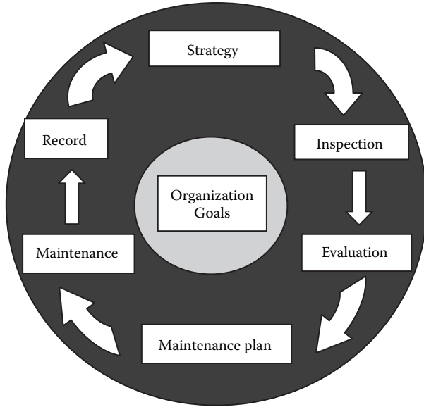
FIGURE 8.1 Structure integrity management system cycle.
