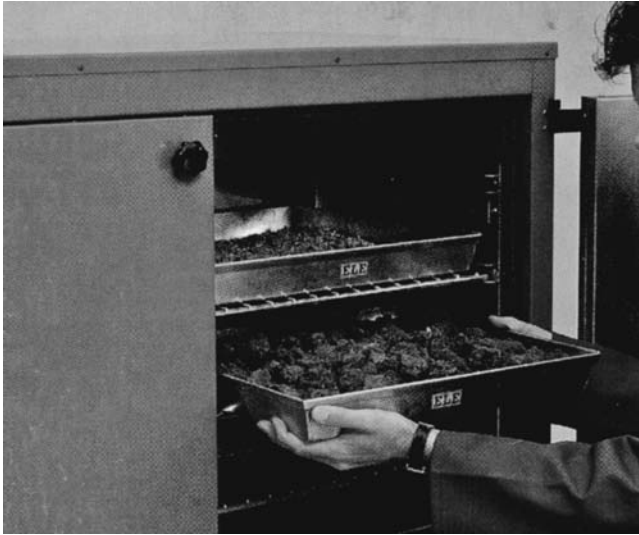
FIGURE 4.7 Oven according to BS1377.
