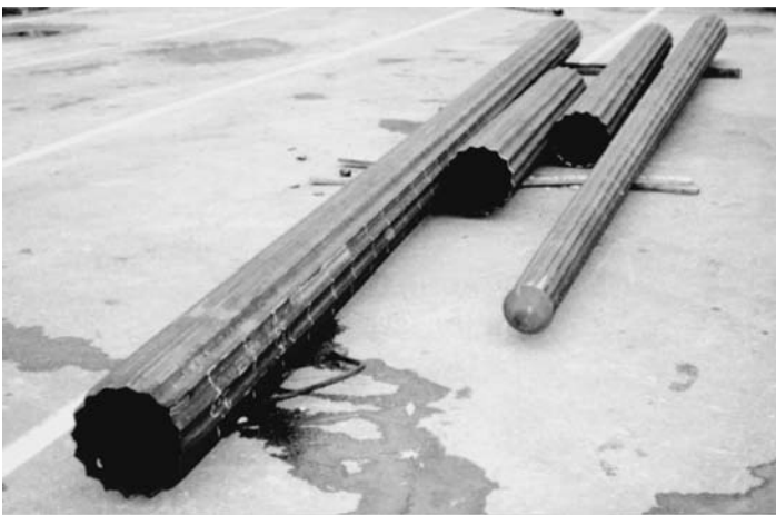
FIGURE 2.55 Raymond shell piles.
