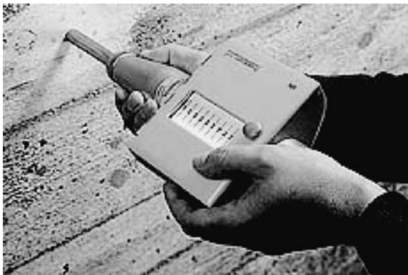
FIGURE 4.16 Testing with rebound hammer.
