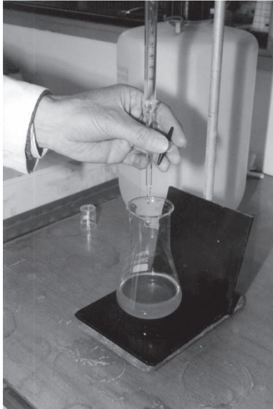
Figure 4.4 Calcium content of the concrete extracts is determined by titration.
