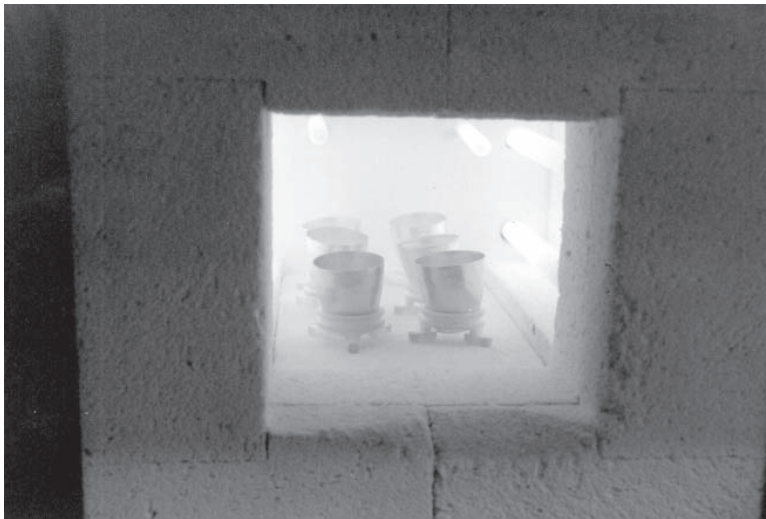
Figure 4.3 Crucibles containing silica are ignited to constant mass at 1100°C.
