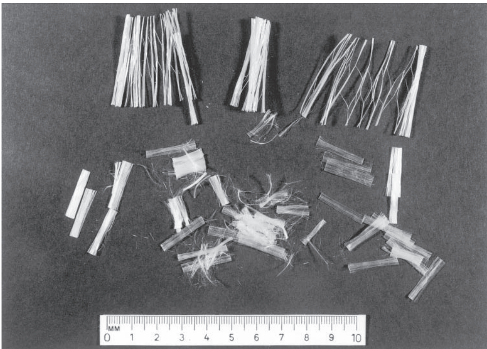
Figure 6.8 Types of fibrillated and monofilament polypropylene fibres.
