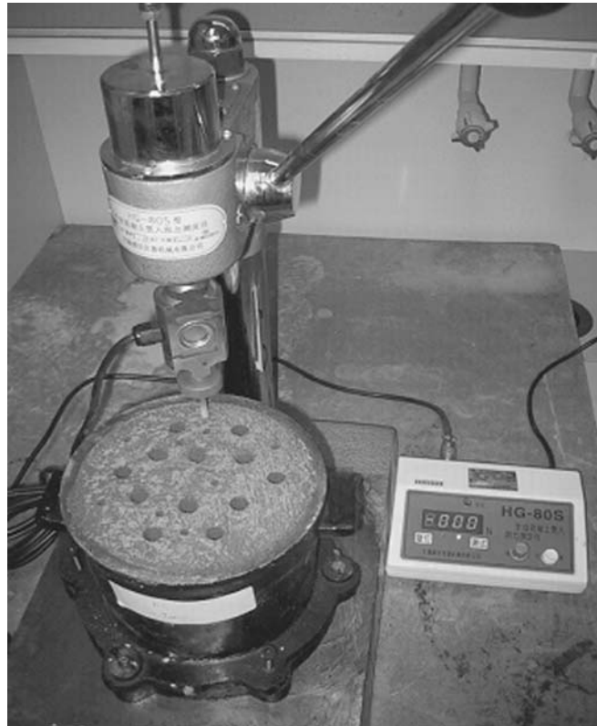
Figure 3-8 Measurement setup of concrete mixture setting time
