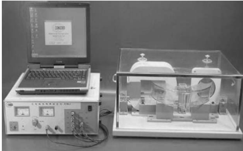
Figure 8-56 A noncontact resistivity test apparatus for cement-based materials
