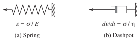
Figure 5-52 Spring and dashpot for modeling viscoelastic behavior
