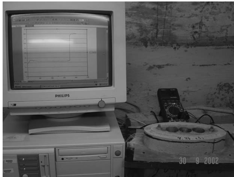
Figure 5-47 Elliptical ring test for constrained shrinkage
