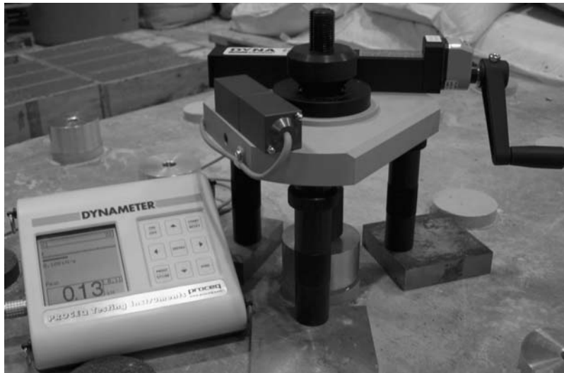
Figure 6-37 Measurement of pull-off strength using a pull-off tester
