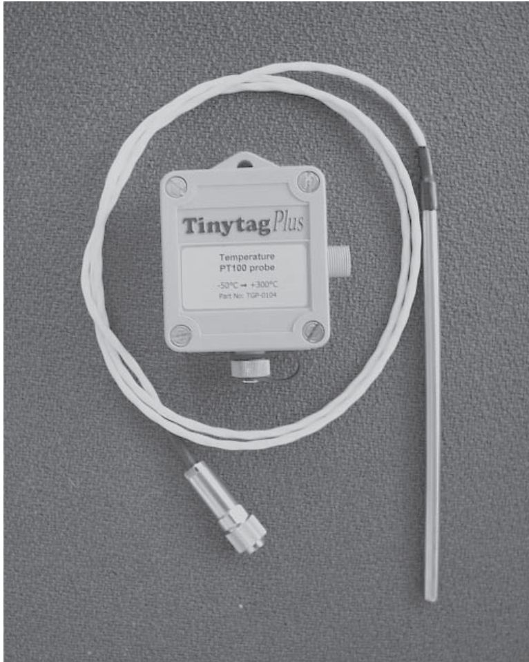
Figure 4.18 Maturity meter (Wexham Development Ltd).
