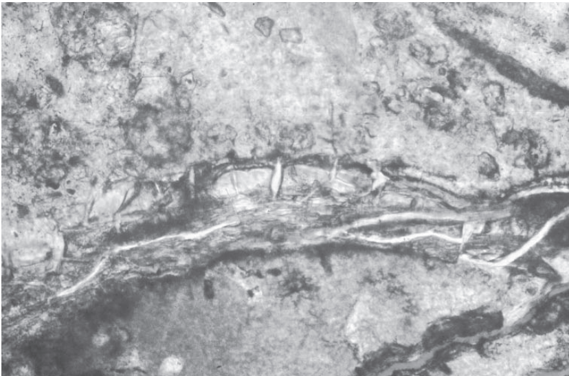
Figure 13.3 ASR gel deposit in a crack remote from the reaction site, under a microscope in thin section. View about 5 mm across.
