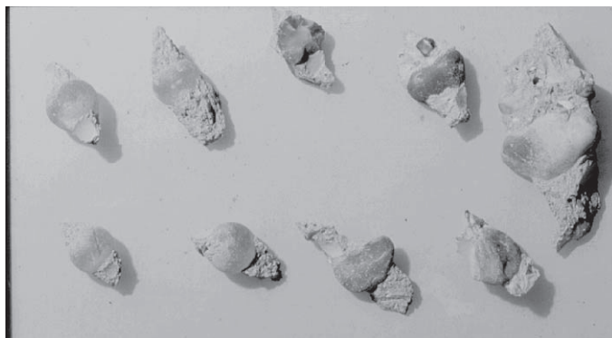
Figure 6.20 Aggregate particles after failure in uniaxial compression.
