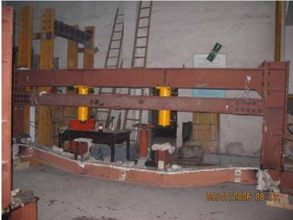
Fig. 7.7 Deflection of the restrained beam
