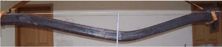
(b) Residual deflection of the restrained column in Test 02
