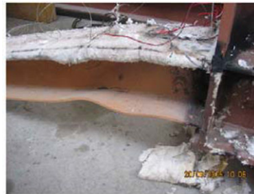
Fig. 7.8 Local buckling of the restrained beam
