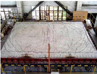
Fig. 9.23 Cracks on the S-2 after the test
