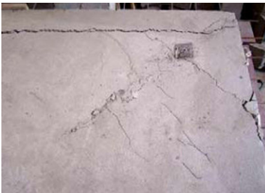
Fig. 9.21 Yield lines at the corner on S-1
