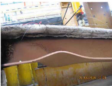
Fig. 7.8 Local buckling of the restrained beam
