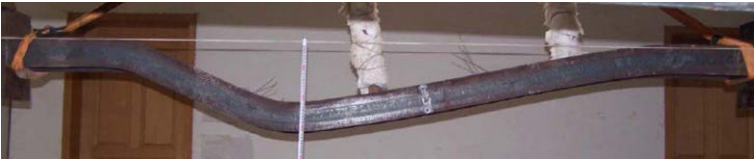
(a) Residual deflection of the restrained column in Test 01
