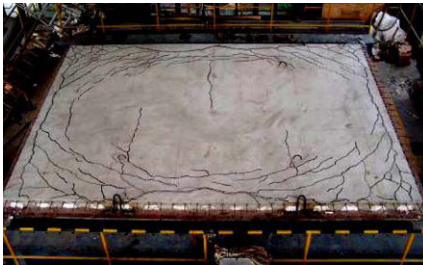
Fig. 9.26 Cracks on S-3 after the test
