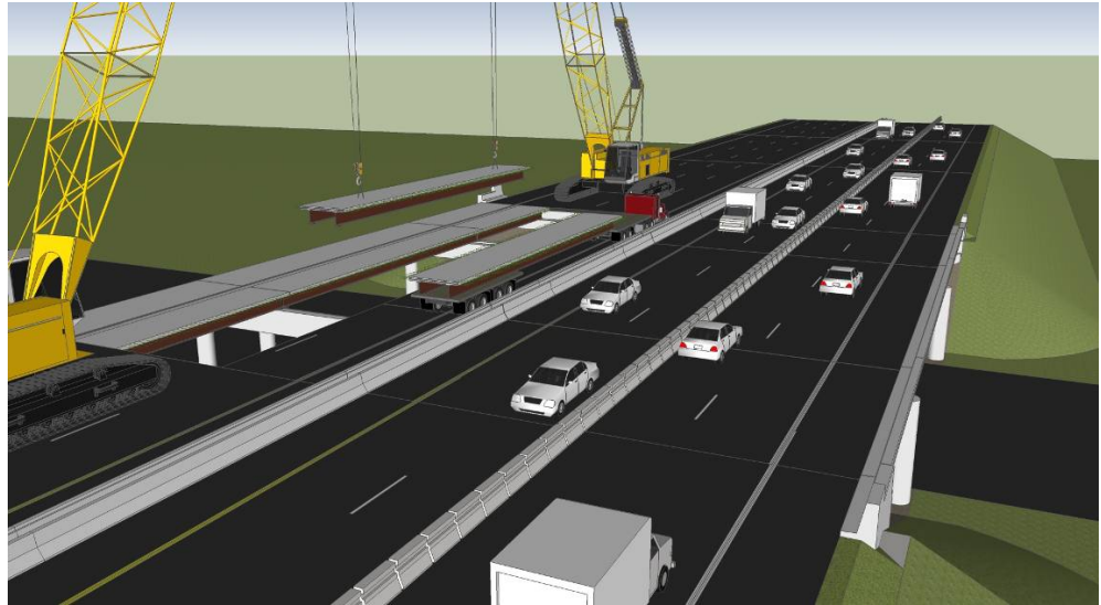
Figure 2.3.1-4 I-93 Superstructure Replacement Concept
