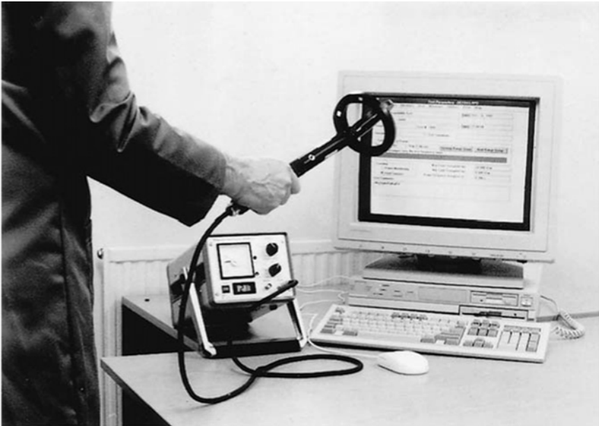
Figure 20.1 Magnetic field portable measurement equipment
