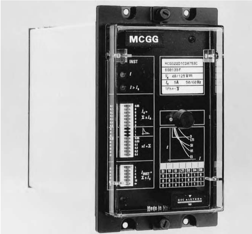
Figure 10.7d Modern microprocessor controlled solid state IDMTL relay – type MCGG. A wide variety of characteristics is available. PSM and TSM settings are configured using the small switches accessible from the front of the relay (courtesy GEC Alsthom T & D Protection & Controls)
