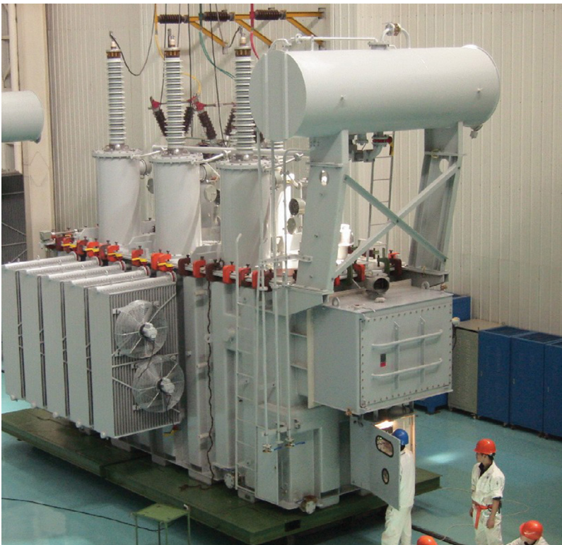
FIGURE 1.17 Large power transformer showing tank and attachments.
