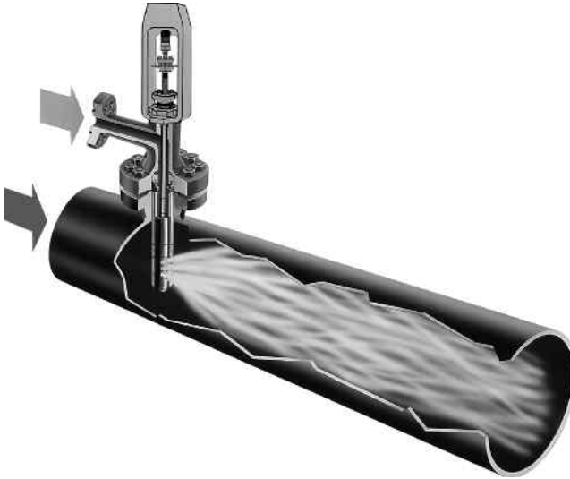
Figure 7.2 Principle of a multinozzle desuperheater. © SPX Flow, reproduced with permission
