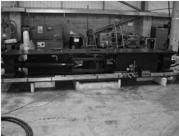
Figure 8.11 Large hydraulic actuator used to modulate 10 m × 10 m damper. Output torque is 1.2 million Nm. © Advanced Actuators Ltd., reproduced with permission
