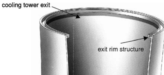
Figure 17: Stabilizing structure at the inner rim side.
