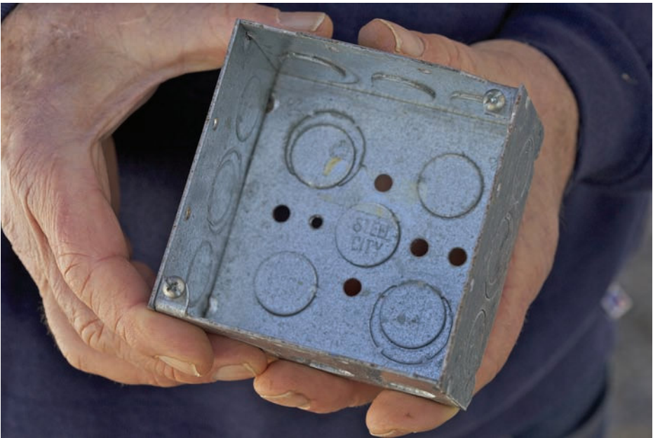
FIGURE 5-8 Large enclosures make for less box fill so that the installation is compliant and there is no chance of conductor damage.
