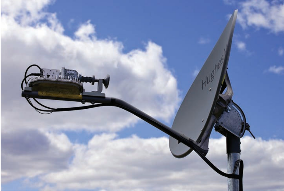
FIGURE 11-1 This satellite dish is stationary, yet it is always pointed precisely at a geocentric satellite.
