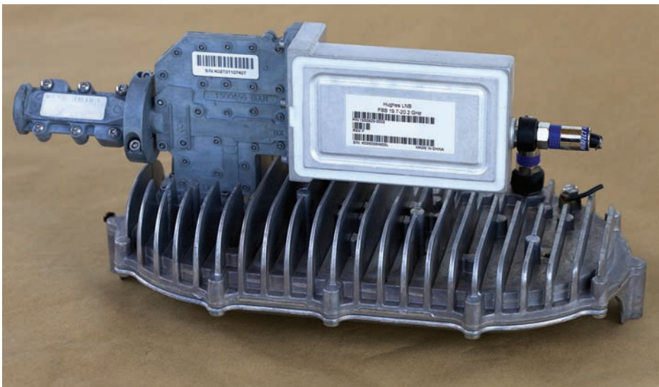
FIGURE 11-2 The low-noise block performs several functions associated with processing a satellite transmission.
