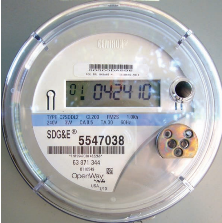
FIGURE 15-3 The new smart meter plugs into the existing meter socket, with no additional wiring required.
