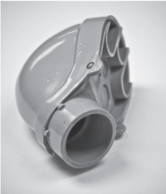
FIGURE 4-7 A weather head, available in metal or PVC, is used at the top end of an aerial service, cable gable, or masthead.
