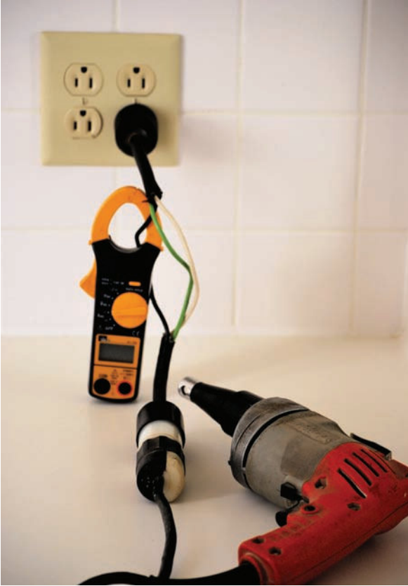
FIGURE 3-1 A clamp-on ammeter reads the current drawn by a portable power tool.
