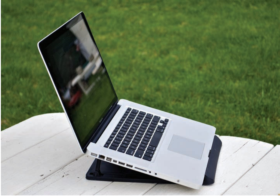
FIGURE 10-7 A stand improves air circulation and is highly recommended for long life of the laptop.
