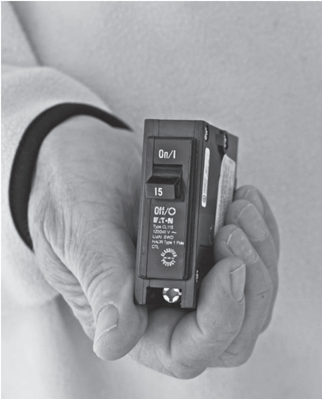
FIGURE 3-4 A 15-amp single-pole breaker used in many 120-volt branch circuits throughout a residence.
