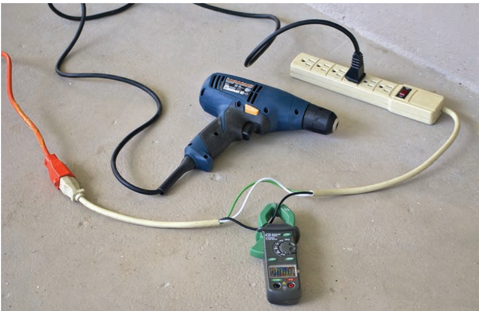
FIGURE 6-7 Clamp-on ammeter measuring current drawn by a portable power tool. Notice the homemade splitter, permitting reading a single conductor.
