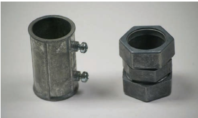
FIGURE G-15 Type EMT fittings: set-screw type at the left for indoor work and compression-type at the right for outdoor work.
