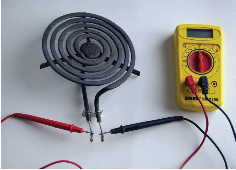
FIGURE 9-3 Checking a burner. It should read low ohms.
