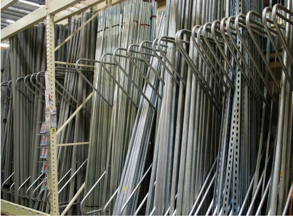
FIGURE 5-24 Type EMT is an excellent general-purpose metal raceway for indoor or outdoor use.
