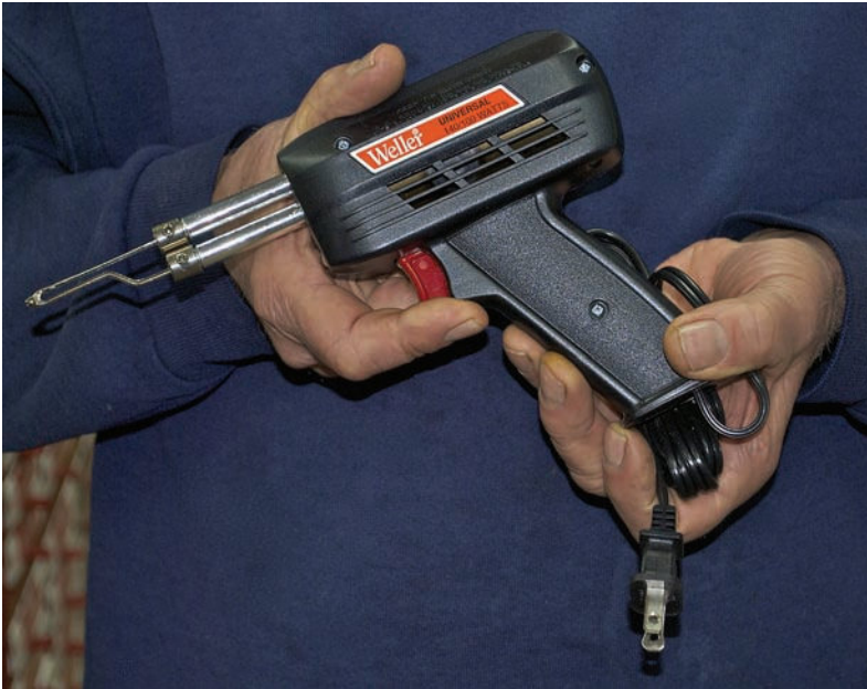
FIGURE 10-5 Pistol-grip soldering iron for large work.
