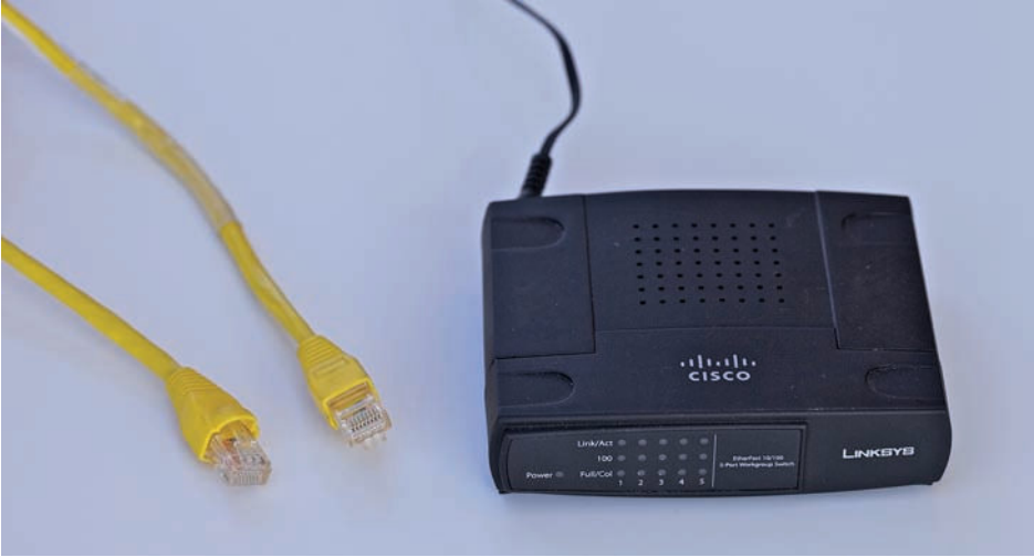
FIGURE 11-8 An Ethernet hub is used where a single feed splits into two or more branches. The wire at the top is an ac power supply. UTP with RJ45 modular connectors plug into a varying number of ports.
