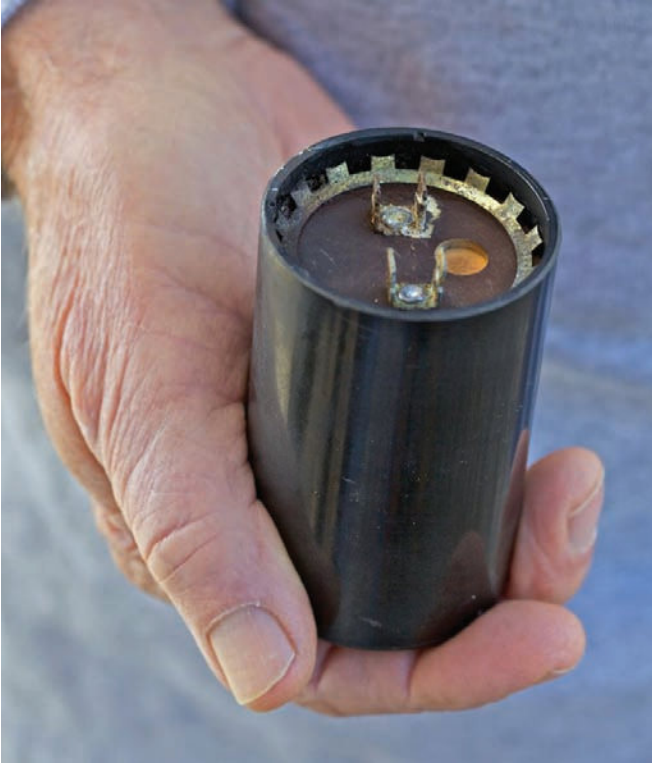
FIGURE 9-5 The electrolytic start capacitor is a frequent offender.
