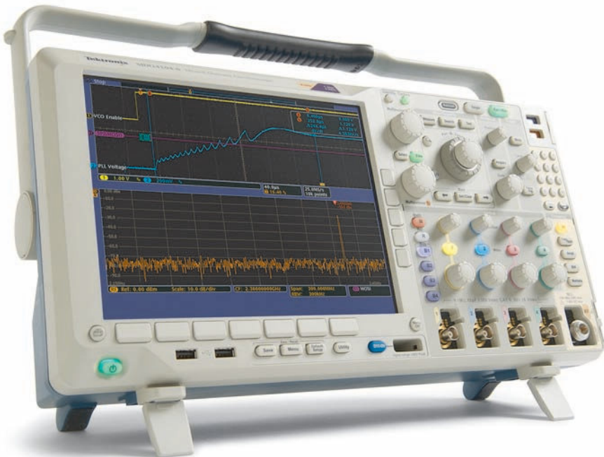
FIGURE 10-3 A digital storage oscilloscope. (Photo courtesy of Tektronix.)
