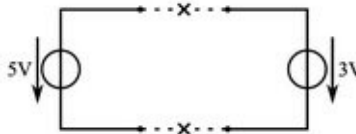
Fig. 3.7: Do not connect ideal voltage sources in parallel.
