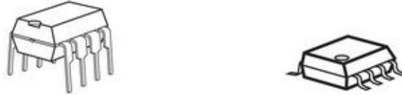
Fig. 6.6: Examples of packages for operational amplifier: DIP-8 (package of \mu A741 OpAmp, left); SOP-8 (right). Package drawings by Infineon Technologies AG.
