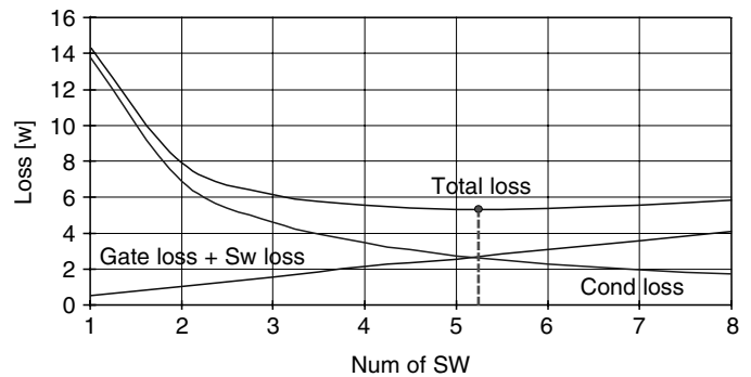
FIGURE 1.11 Switching Loss, Gate Drive Loss, and Conduction Loss of an IRL3803 Versus a Parallel Switch Number ( V_{in} = 5\text{ V} , f_s = 300\text{ kHz} , and I_{load} = 50\text{ A} )
