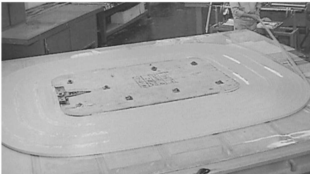
FIGURE 3.20 Pancake winding during winding process.
