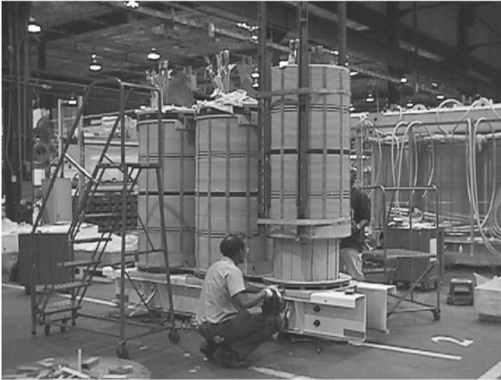
FIGURE 3.16 Concentric arrangement, outer coil being lowered onto core leg over top of inner coil.
