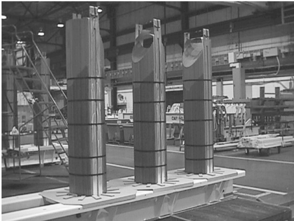
FIGURE 3.13 “E”-assembly, prior to insertion of top yoke.
